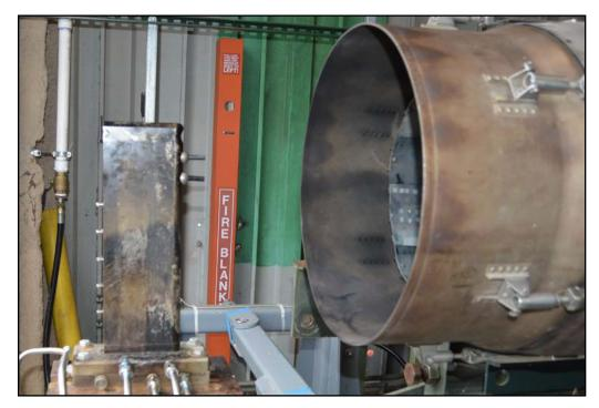
A sample of additively manufactured silicon oxycarbide (SiOC) material is tested at Arnold Air Force Base. The testing was conducted as part of a Cooperative Research and Development – Material Transfer Agreement between Air Force Research Laboratory Aerospace Systems Directorate and HRL Laboratories. (AF Photo.)
