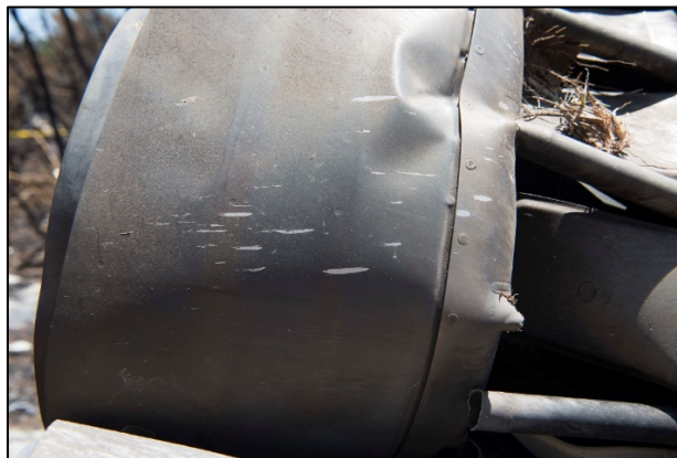
Figure 2: Aluminum Splattering on the Ejector Assembly (Tab J-19)
