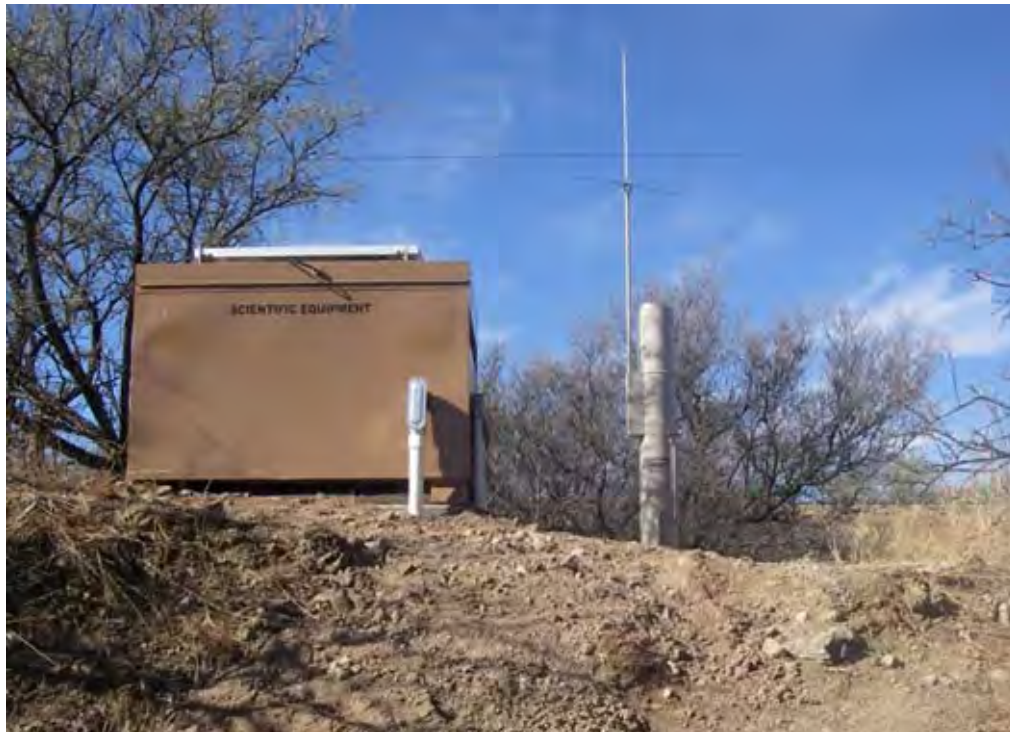
Figure 2. Standpipe Housing with ISCO Enclosure (Davidson Canyon installation)
