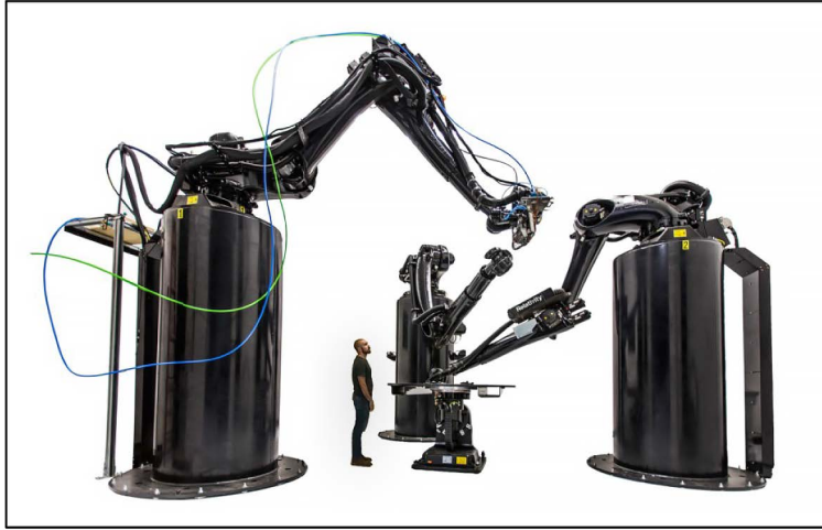
Figure 7. Robotic AM system. (Reproduced from Relativity Space, accessed 20 April 2018, https://www.relativityspace.com/stargate .)
