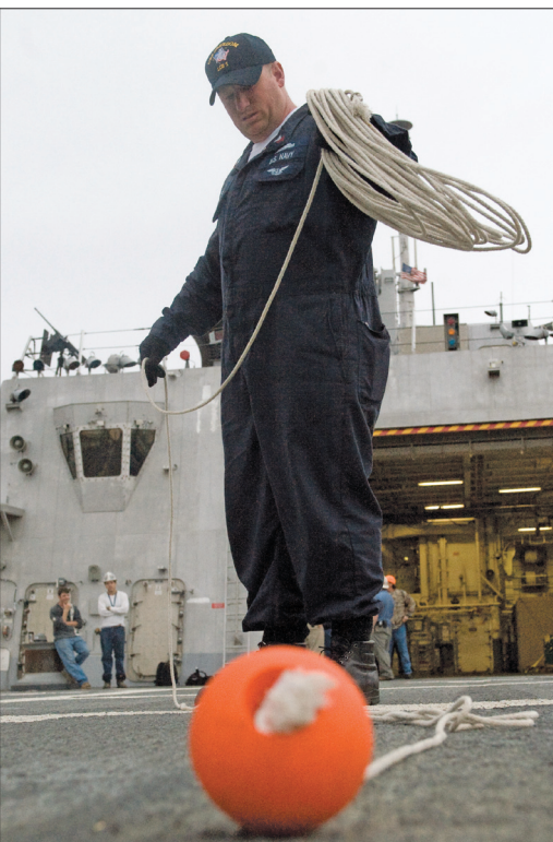
▲ Smith prepares the messenger line for line handling prior to getting underway aboard Freedom .
