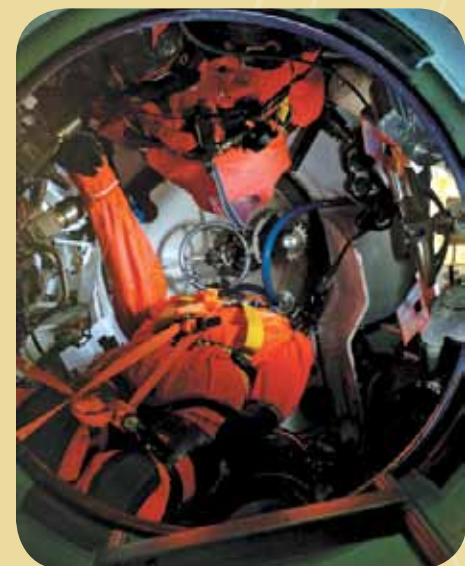
▲ Virginia ’s Submarine Escape Immersion Equipment is designed to facilitate safe escapes from as deep as 600 feet.
