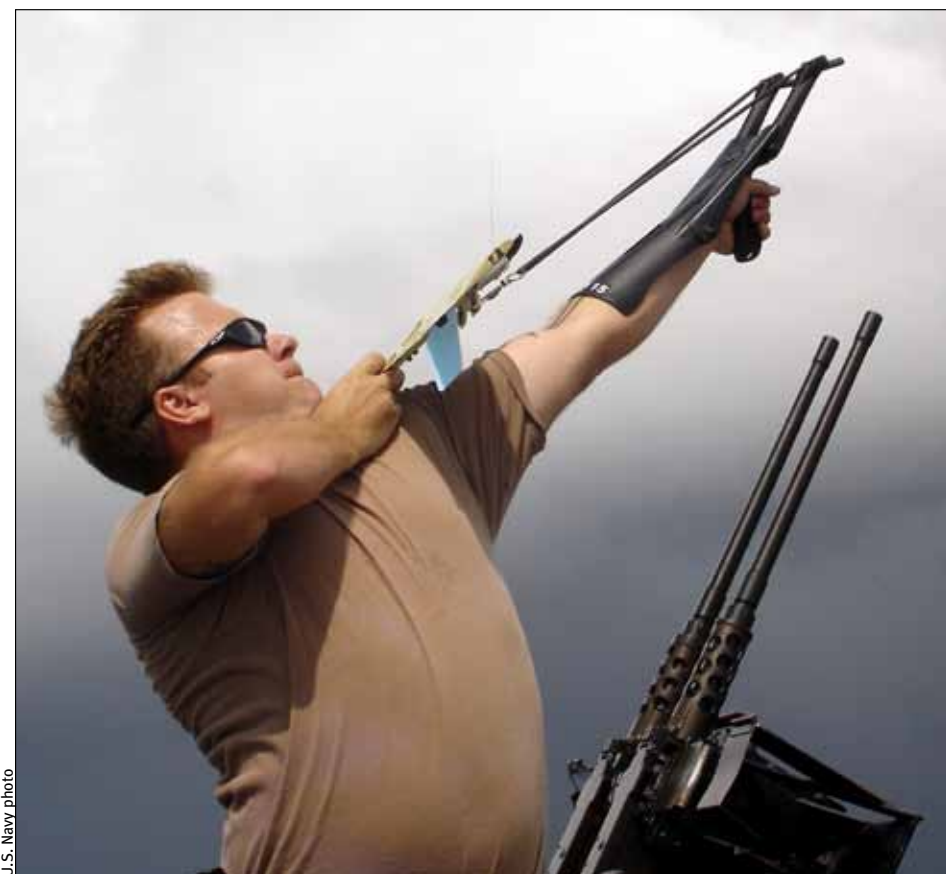
▲ A turret gunner launches a Swift Unmanned Aerial Vehicle (UAV) from the top of a Humvee with a specially-designed slingshot. SEAL Teams use UAVs to help scout out rugged terrain and urban areas in real-time.
