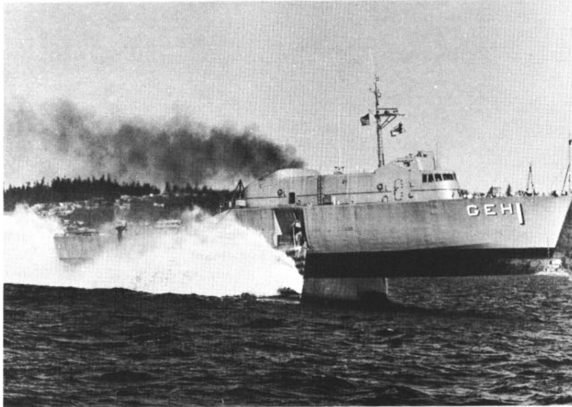
PATCHING OUT—The Navy's Plainview , the world's largest hydrofoil, churns up the water of Puget Sound. The hydrofoil is capable of speeds over 40 knots.
