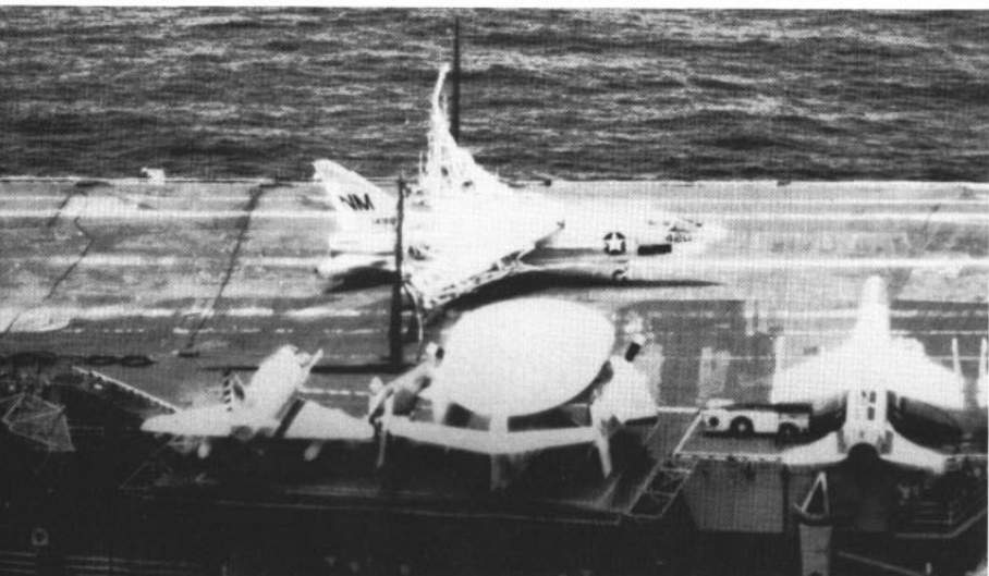
HOME SAFE— Crusader with stuck landing gear makes barricade arrested landing aboard Ticonderoga (CVA 14).
