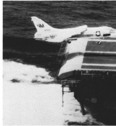
HOME SAFE— Crusader with stuck landing gear makes barricade arrested landing aboard Ticonderoga (CVA 14).
