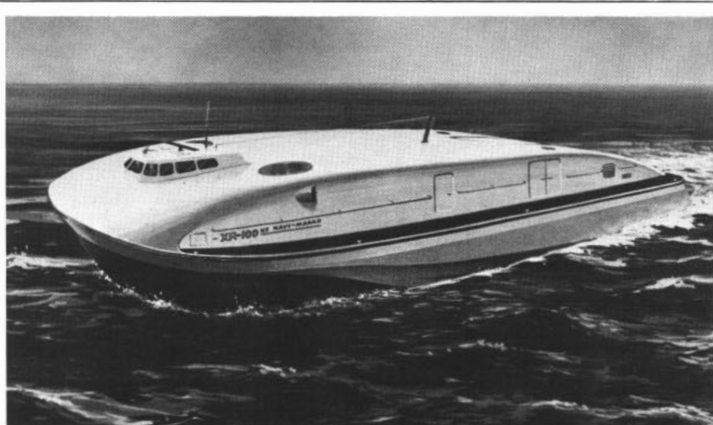
ON CAPTURED AIR—Artist's conception shows one of several versions proposed for a 90-ton Surface Effect Ship (SES) experimental test craft. It uses a modified captured air bubble concept, wherein the air cushion is contained between two solid sidewalls. Goal is 80 knots or higher on smooth seas.
