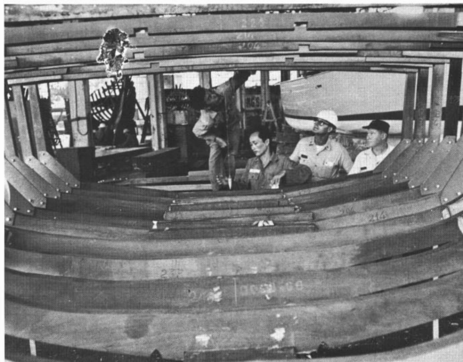
READY TO SEARCH —Three new junks await sea trials and then will join coast Junk Force. Below: Vietnamese workers aline rib as U. S. advisors look on.
