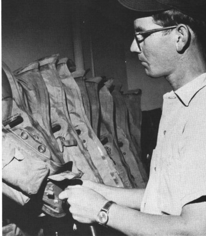
JACKET TESTER —Aircrew Survival Equipmentman David Morea inflates jackets for 24 hours and then tests for leaks.
