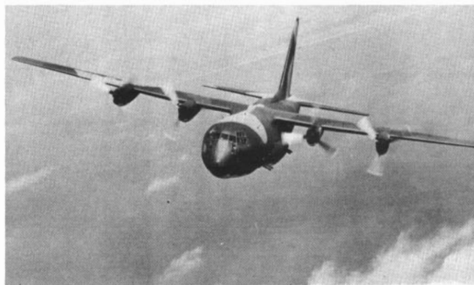
VERSATILE —The AC-130 gunship combines reconnaissance and strike capabilities in the same aircraft.
