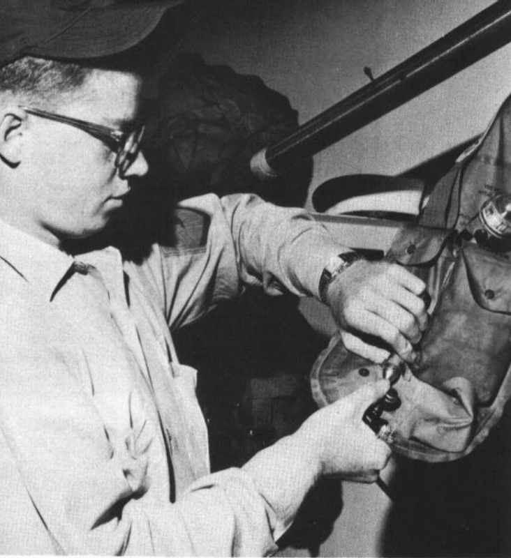
PETTY OFFICER 3rd Class James Hobby installs a CO2 cylinder in a life jacket. Rt: Parachutes being dried.
