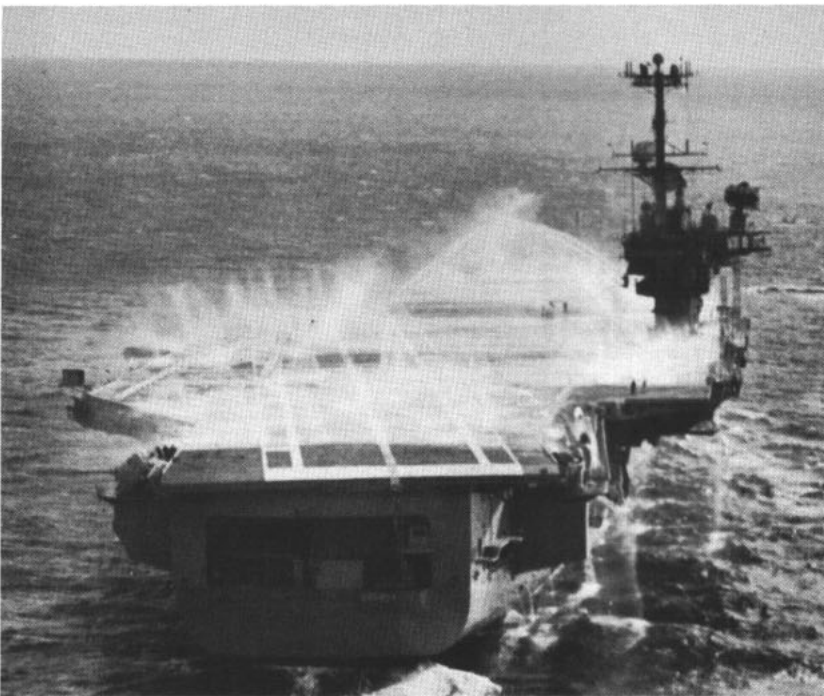
WATER WASHDOWN —Aircraft carrier USS Independence (CVA 62) floods her deck as she pumps 'light water' through her water washdown system during a series of firefighting tests aimed at finding better means to control flight deck fires.
