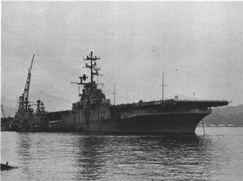
HANG OVER—USS Princeton (LPH 5) uses her anchor to ease the strain as she ties up at Subic Bay to pier that is some 460 feet shorter than her length.
