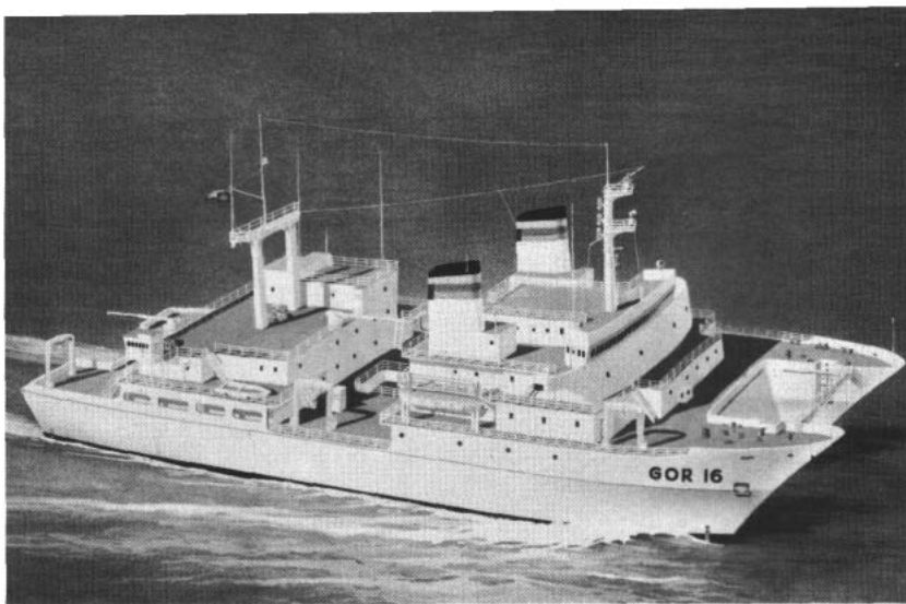
SEA SEARCHER —Artist's conception shows new Navy oceanographic research ship. Catamaran design will provide a stable platform for scientific studies.
