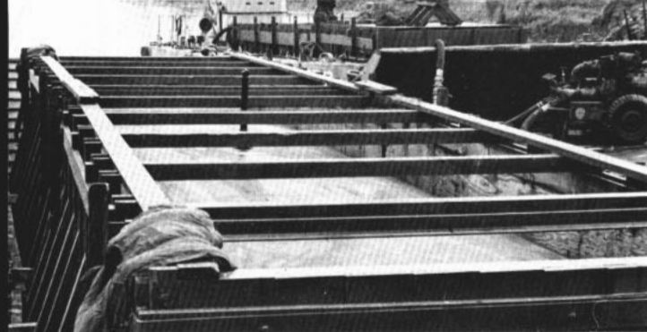
CRIB supports inflatable container aboard LCM. Rt. : LCM is converted to a tanker with this container.
