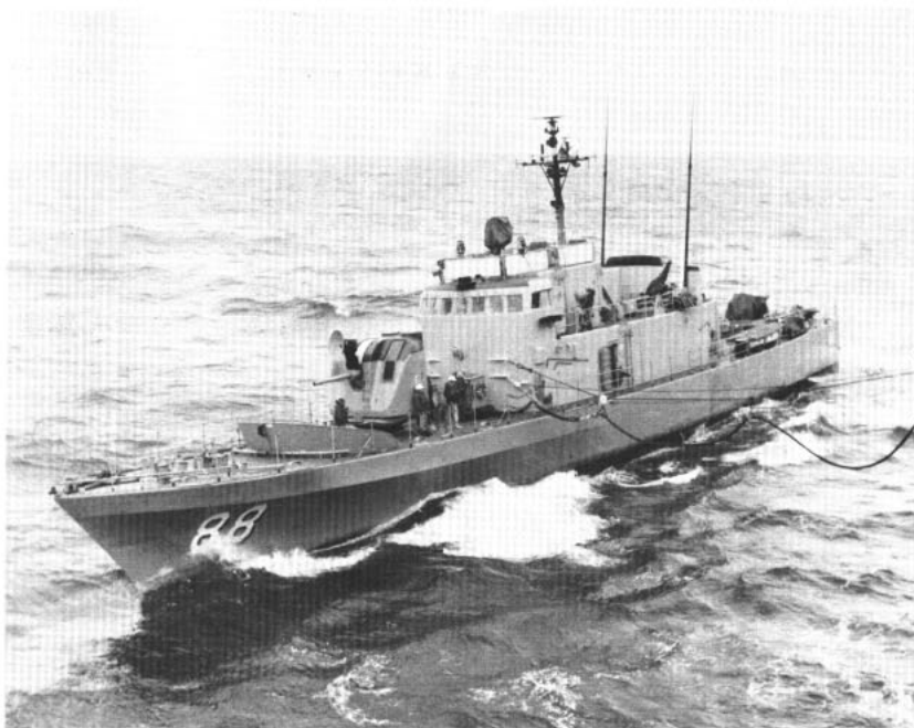
FAST FUELER —Jet-propelled gunboat USS Crockett (PG 88) is refueled while underway at sea during a recent trans-Pacific cruise from Hawaii to Guam.
