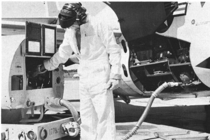
TRANSFER —Jet's oxygen converter is filled with LOX at NAAS.
