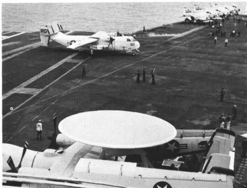
COMBAT COUSINS—C24 Greyhound cargo plane taxis after first landing on carrier in combat zone. In foreground is E2A Hawkeye early warning radar plane.
