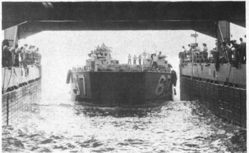
SWALLOWED—YFU enters well deck of LSD for supply run to Dong Ha.
