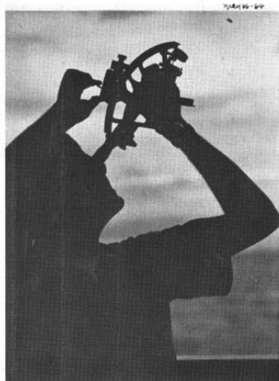
SILHOUETTE STAR SHOOTER —Officer of the Deck takes star reading on sextant to figure ship's position.
