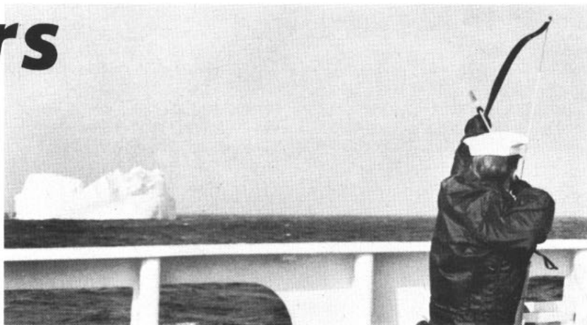
SHOOT AND DYE—Arrow with dye marker on tip marked bergs for identification. Below: Oceanographic vessel Evergreen has bow for breaking icebergs.
