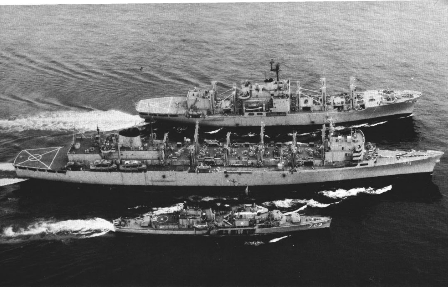
FAST SERVICE — USS Sacramento (AOE 1) refuels USS Mars (AFS 1) and USS Walke (DD 723) during Western Pacific deployment. Sacramento and Mars use UH-46C helicopters for vertical replenishment, accompany fast task forces.
