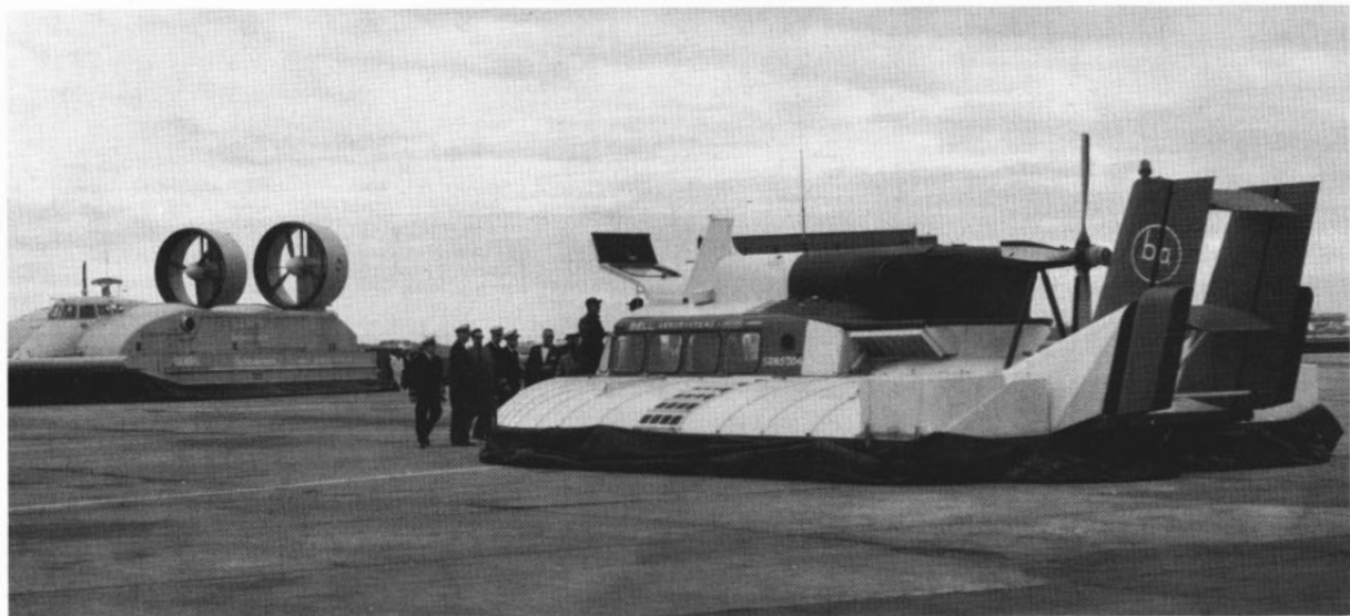
HIGH AND DRY—Two of GEMs tested by OpTevFor rest ashore during the evaluation of the air cushion systems.
