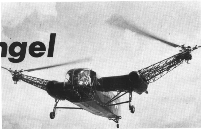
TWO-TIMER—World's largest (back in 1946), also Navy's first twin engine job, was used as research vehicle. Below: Early demonstration in air-sea rescue.
