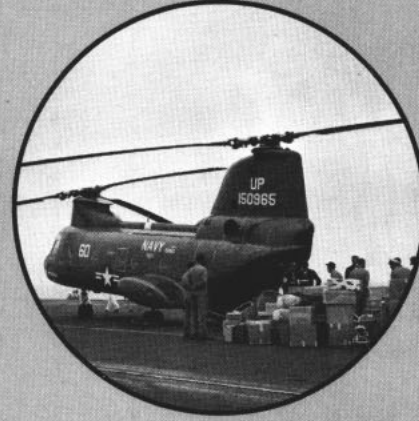
NO KITCHEN SINK? —Wide assortment of cargo demonstrates carrying capacity of H-46 Sea Knight, which can haul up to 8000 pounds.
