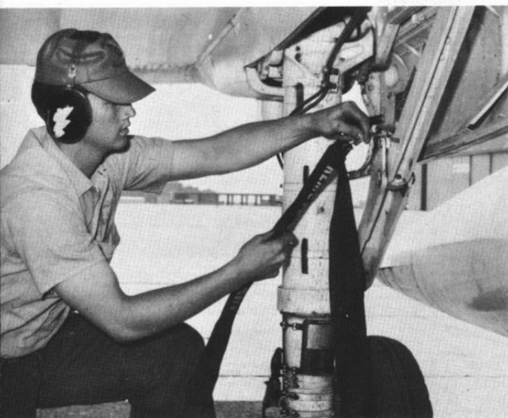
PLANE CAPTAIN pulls main landing gear safety pins prior to flight. Right: Parachute rigger maintains flight gear.
