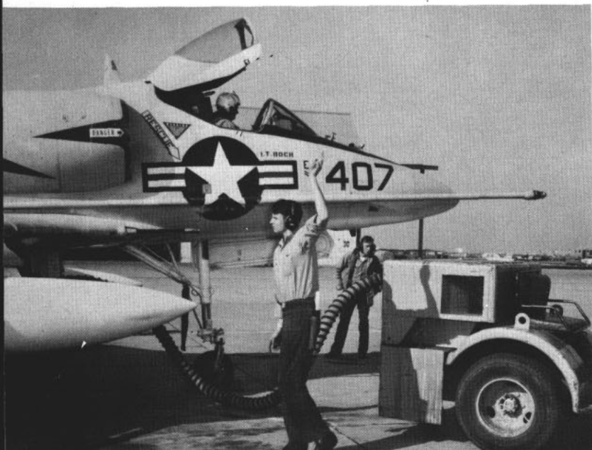
AIR TURBINE hose stiffens with pressure of air used to start jet engine. Rt: Pilot's name is stenciled on plane.
