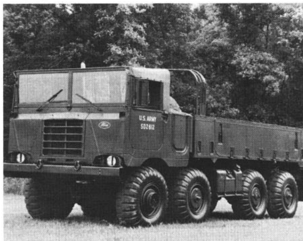
LIGHTWEIGHT —XM656 truck is two tons lighter than present Army five-ton truck, can be transported by air.
