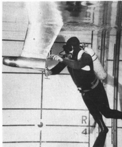
FROGMAN makes adjustment on model of waterjet propulsion unit. Test of unit showed system could drive Navy ship at speeds of 76 knots.
