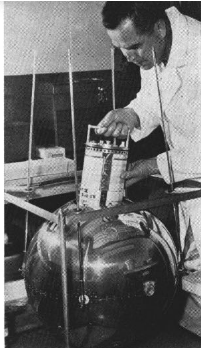
IGY SATELLITE program included Navy's development of Vanguard rocket and satellites. Here, Vanguard is readied and instruments are inserted.
