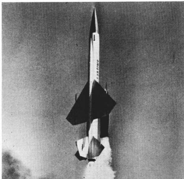
STRAIGHT UP —An Air Force Bomarc, long-range air defense interceptor guided missile, goes after target.
