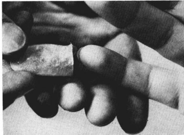
NYLON PRINTS —Army has developed three dimensional finger printing, using nylon compound spray to cast.
