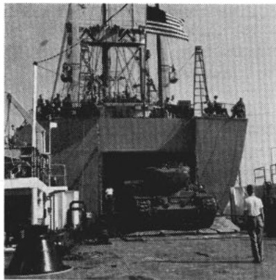
ROLL OFF —Tank rolls off USNS Comet onto flat top deck of Army's beach discharge lighter, Lt Col John U. D. Page, for landing on the shore.
