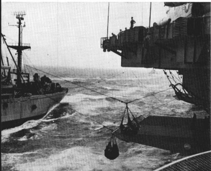
ALL HANDS JOB—Transferring supplies by high line underway at sea takes team work from bridge to hold.
