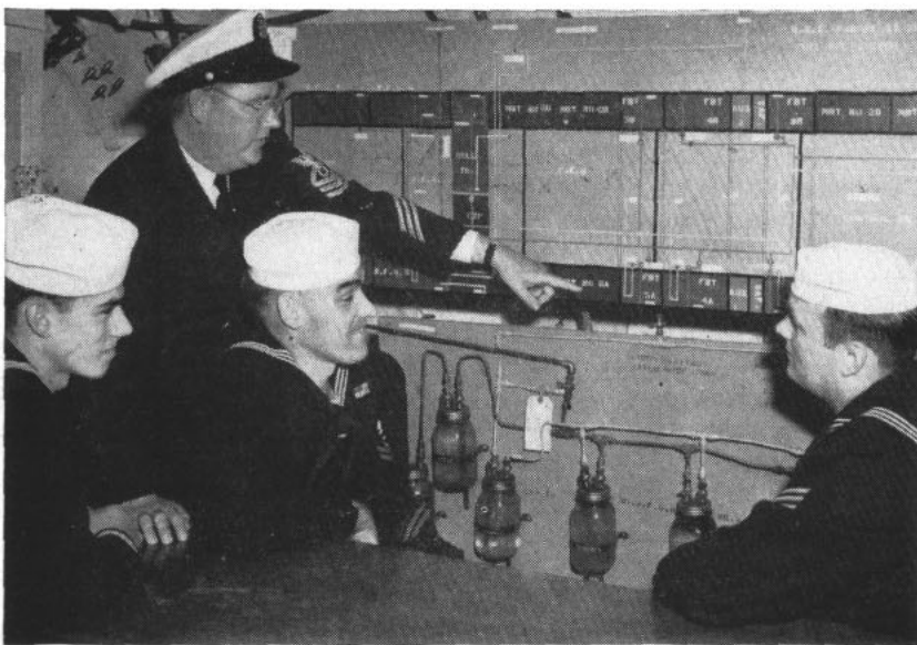
SKULL SESSIONS on dry land come before a Reservist is sent to sea for actual shipboard training. Chief checks out his men on a submarine's fuel oil system.
