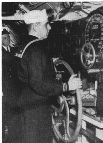
SURFACING SUB glistens in the sun (left). Top: Reservist manning stern plane watches depth indicator during dive. Right: Controllerman cocks ear for order.
