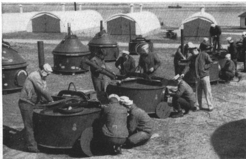
NEXT DAY it is work as usual as trainees turn once more to solving the intricate mechanisms of explosives like these Mark 51 controlled mines.
