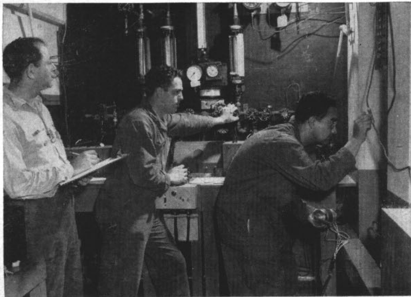
OBSERVING actual operation of a ramjet engine in simulated flight, Navy trainees peer into test chamber. Man, left, checks dials while man, center, regulates fuel. Right: trainee tests equipment he will use; instructor looks on.
