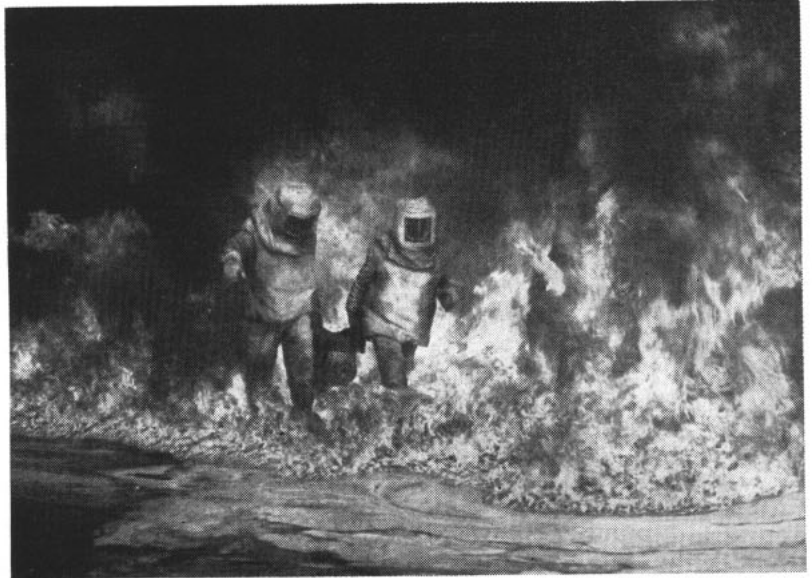
HOT POPPAS emerge unscathed from raging gas and oil fire, dragging a 'victim' with them. In this test, temperature reached a torrid 2100 degrees.
