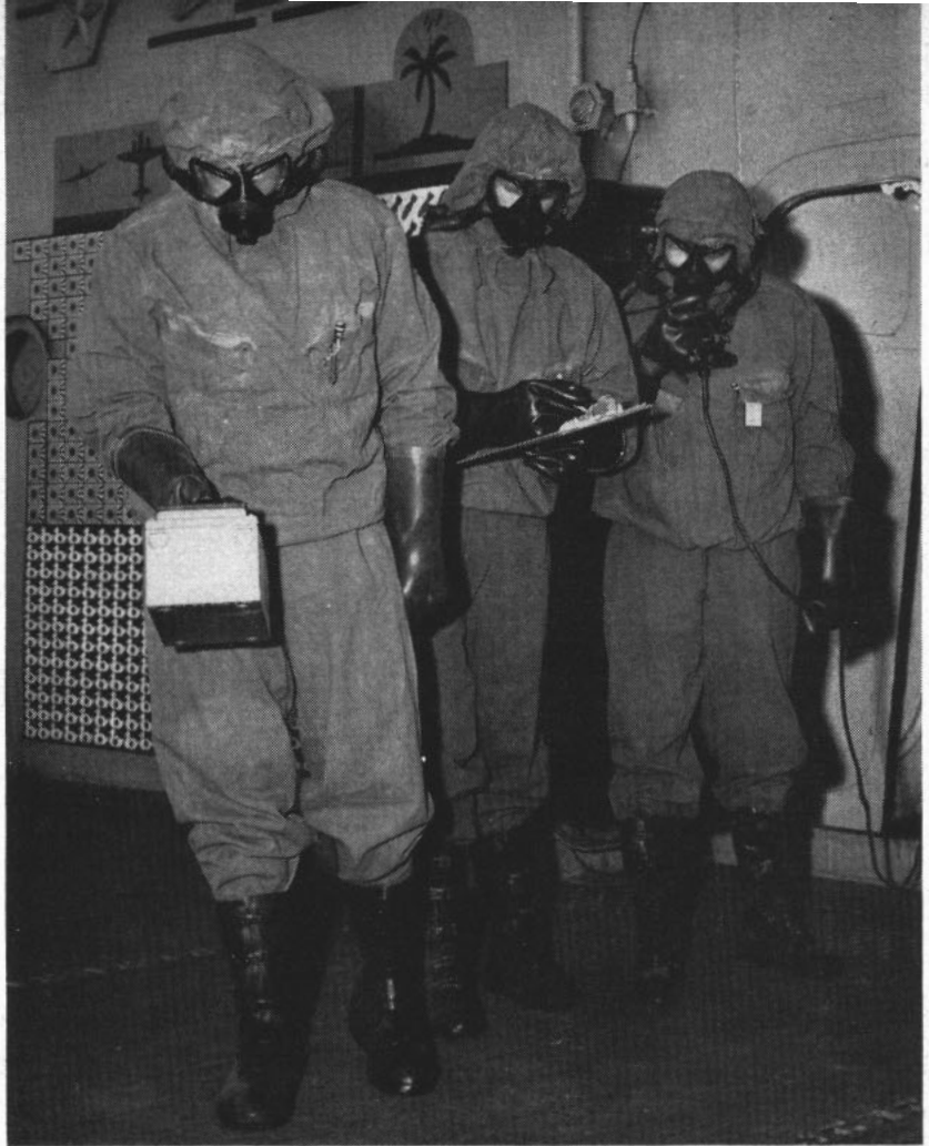
SURVEY PARTY steps out onto the weather deck. The intensity of radiation from 'hot' planking is determined by radiac instrument in man's right hand.
