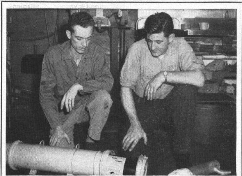
SAVVY shipmates Robert VanBeck TSgt, USMC, and Robert Barr, ME1, USN, designed film container to be dropped from Corsair bomb racks.
