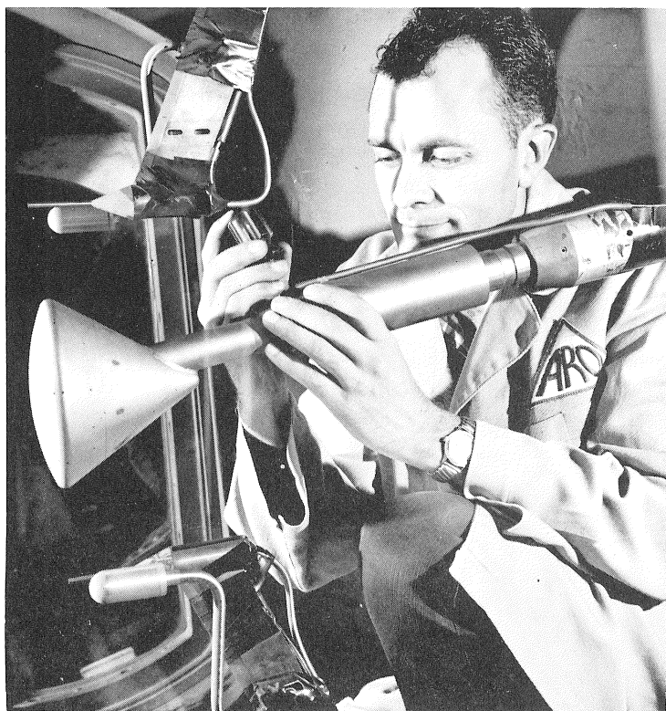
MACH 20 RE-ENTRY TEST – for a scale model of the Apollo command module was conducted in the 100-inch hypervelocity wind tunnel in the von Karman Facility. ARO technician J.W. Helton adjusts the model support.
