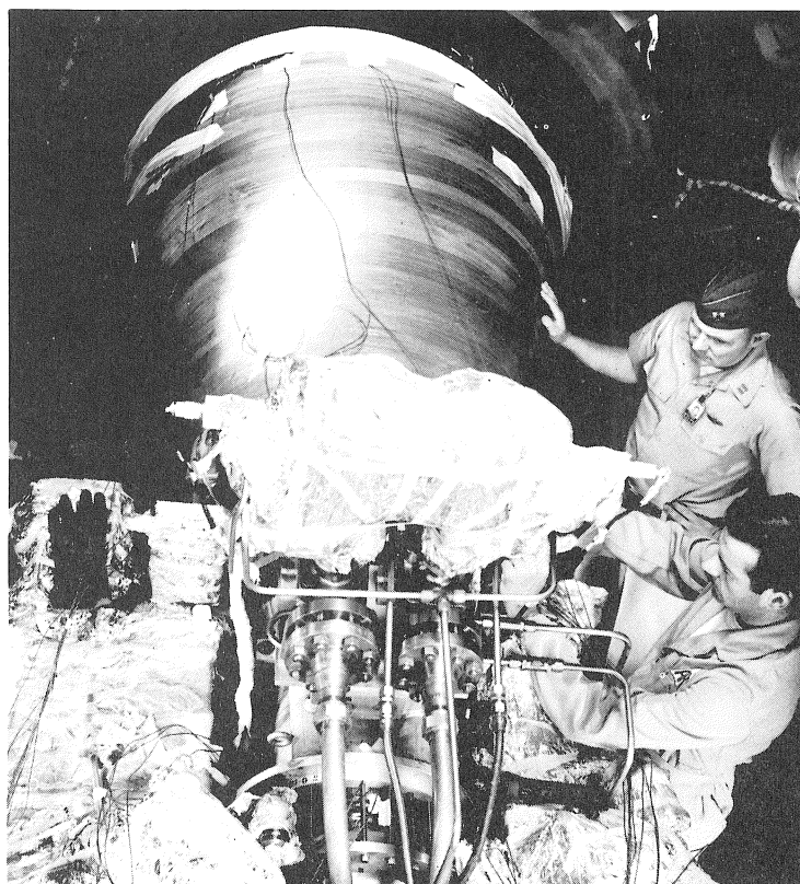
ASCENT ENGINE – for LEM module being prepared for high altitude test in Rocket Test Facility. Capt. E.C. Westwood watches ARO technician D.L. Easley make final adjustments.
