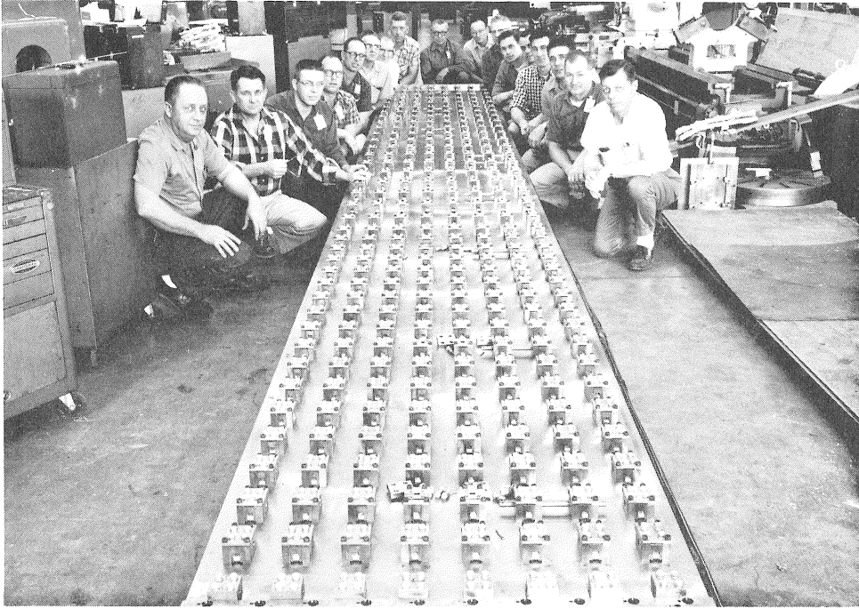
BIG JOB, HIGH PRECISION —Grouped around the spare flexible nozzle plate recently completed by the von Karman Facility Shop are the men responsible for the job: (from left) J.B. Baker, J.M. Johns, E.M. Yother, J.L. Parker, R.O. Angel, Jr., W.J. Gravlee, G.L. Cleveland, J.L. Wiseman, K.J. Ramsey, N.H. Smith, W.D. Brackman, E.W. Pross, E.K. Wood, J.E. Rogers, J.E. Brazelton, Lavoy Kilgore and R.G. Watts.
