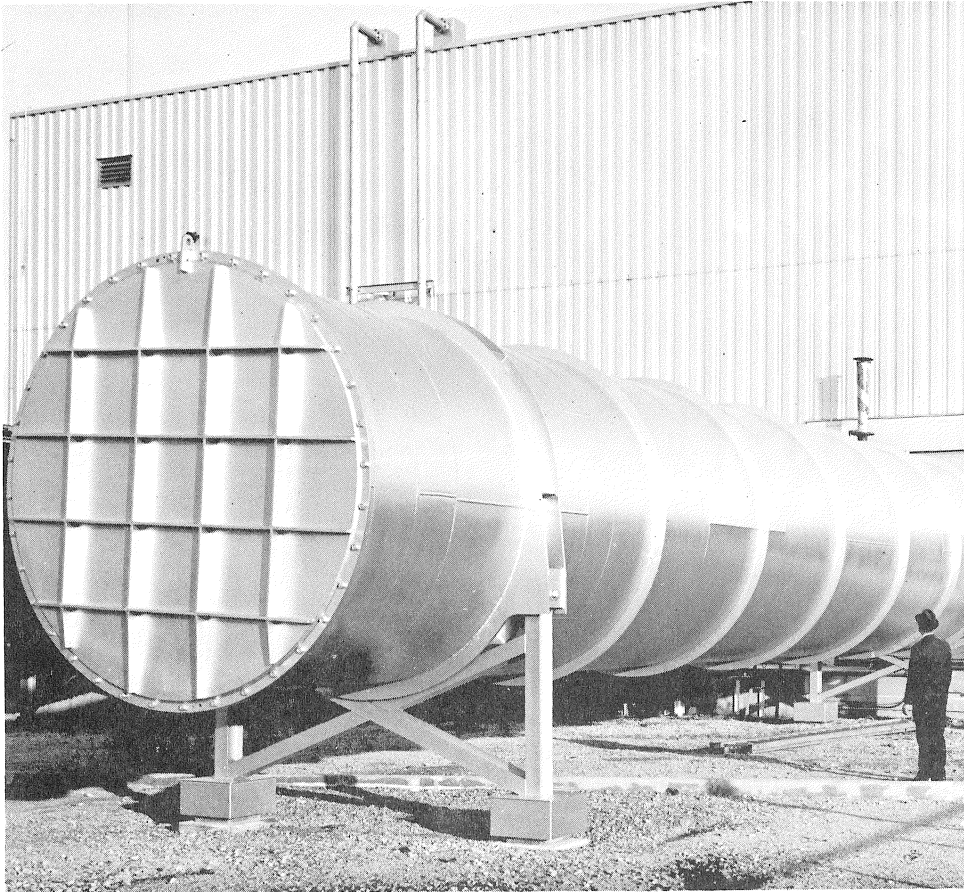
ADDITIONAL LENGTH increases vKF run time, provides longer period of usable flow; thus, more data from a single firing.
