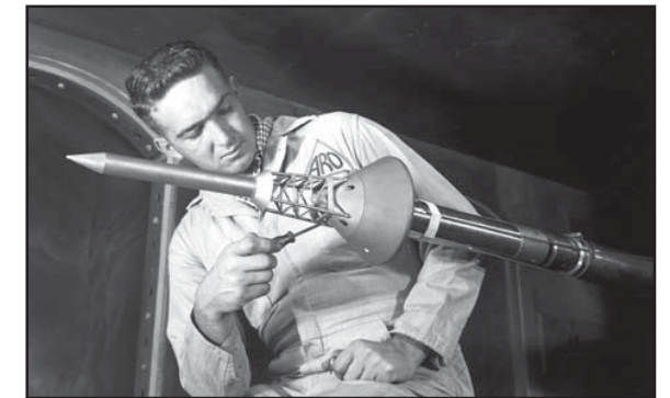
AEDC engineers performed detailed tests on a number of facets of NASA’s Apollo program, including aerodynamic testing of this scale model of the Apollo three-man capsule with its escape tower in 1962. Later tests established the need for canard control surfaces at the apex of the escape rocket.
