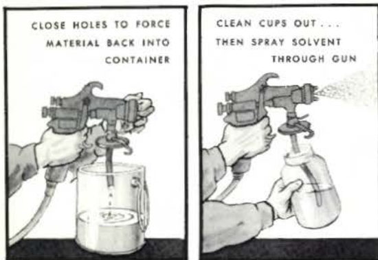
Fig. 47. Steps in cleaning a container type gun.
