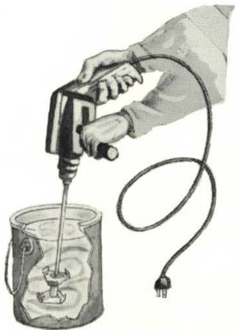
Fig. 4. Paint mixing attachment for electric hand drill.
