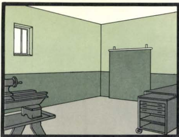
In shops and laboratories, use Principle O, No. 1 Light Green walls and No. 2 Medium Green trim and dado.
