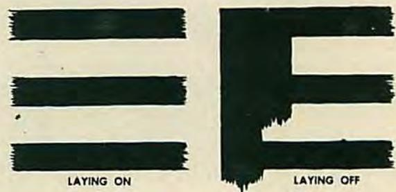
Fig. 9. Proper method of applying paint.
