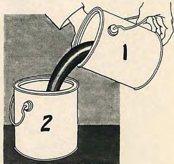
Fig. 2. Pouring off the top liquid.
