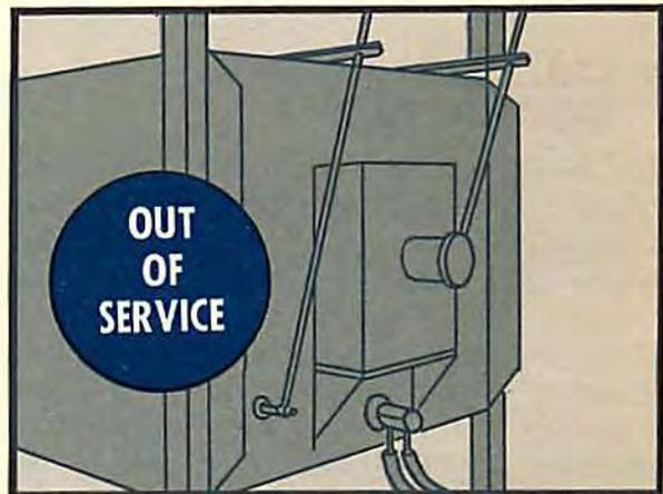
Out of service signs, in blue, shall be used for equipment, boilers, elevators, *shut* out down for repair.
