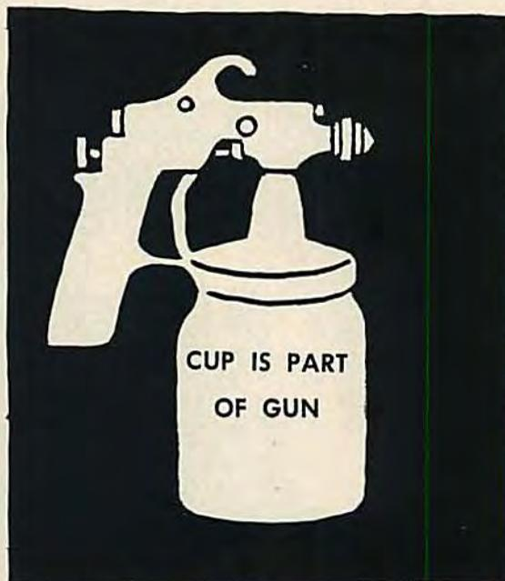
Fig. 13. Attached container type.
