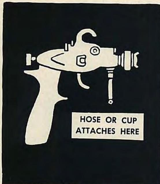
Fig. 12. Separate container type.
