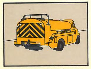
Gasoline trucks, mules, tractors, transporters used on air fields shall be No. 14 Brilliant Yellow.
