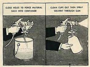
Fig. 42. Steps in cleaning a container type gun.
