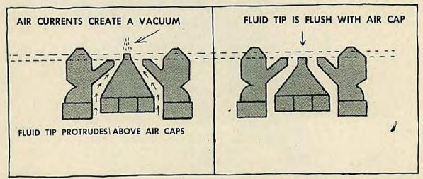
Fig. 26. Suction or gravity feed cap.
