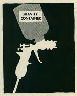
Fig. 20. Gravity feed type.
