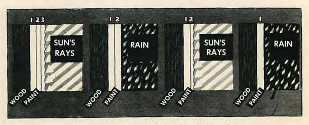
Fig. 47. Progress of chalking with outside paint.
