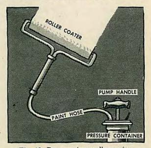
Fig. 46. Pressure type roller coater.
