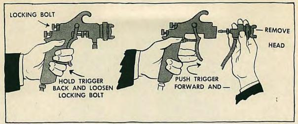
Fig. 25. Method of removing spray head from gun body.
