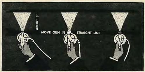
Fig. 38. Proper method of spraying.
