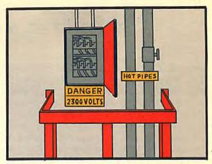
Orange should mark hot pipes, exposed electrical connections, and all cutting, crushing or shocking dangers.
