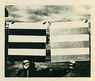
Fig. 4. Contrast Ratio of Pattern: left pattern black and white. Right pattern International Orange (Fed. Color No. 1205) and white. Film and filter selected to show brightness contrast as seen by human eye at short ranges.
