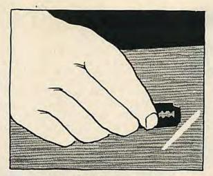
Fig. 4. Patch is scraped level.
