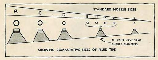
Fig. 28. Fluid tips come in different sizes.
