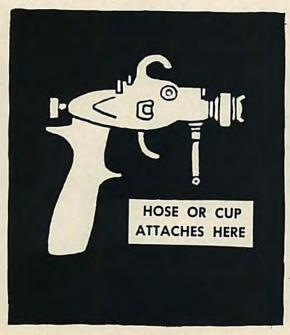
Fig. 12. Separate container type.
