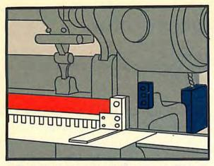
No. 18 International Orange shall be applied on or near the hazardous parts of shears, knives, rollers, gears.
