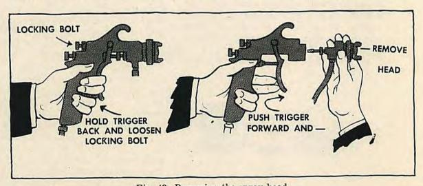
Fig. 43. Removing the spray head.
