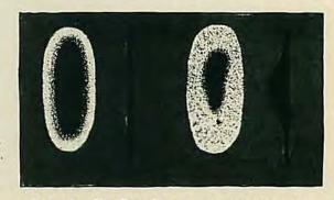
Fig. 41. Good and poor spray patterns.
