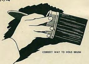
Fig. 7. Brush is held firmly, as shown.
