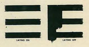
Fig. 9. Proper method of applying paint.
