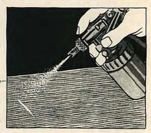
Fig. 6. Clear lacquer is sprayed.
