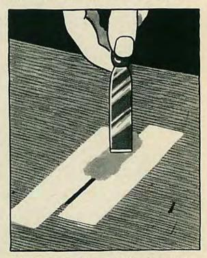
Fig. 3. Application of shellac to scratch.
