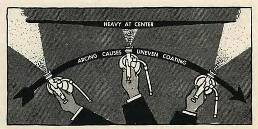
Fig. 39. Improper method of spraying.
