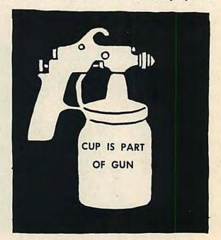
Fig. 13. Attached container type.
