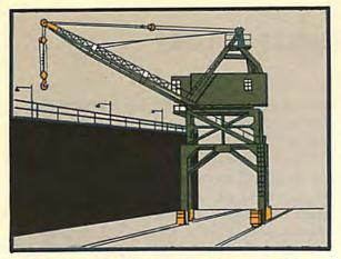
Cranes and shipway structures shall be No. 12 Spruce Green with safety marking in No. 14 Brilliant Yellow.
