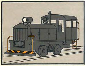
No. 20 Medium Gray shall be used for locomotives, railway cars, railway and automotive cranes and winches.
