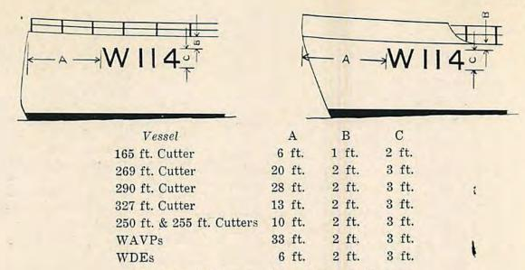
Dimension A is measured in a fore and aft plane. All other measurements are along the hull. Dimension B is measured from main deck downward.
