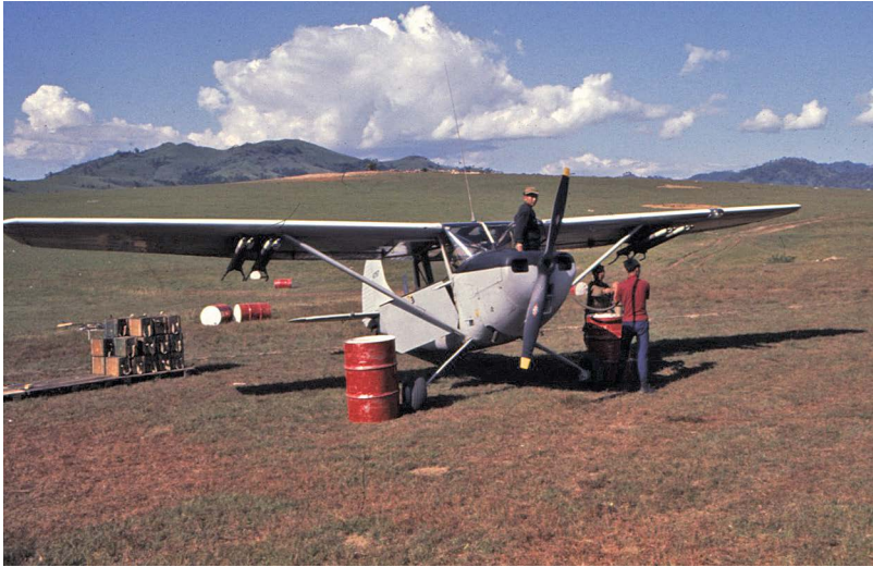
Above: A Raven O-1 being hand filled with aviation fuel from 55-gallon drums, somewhere on the PDJ . (Photo courtesy of John Garrity collection via William E. Platt.) Below: The 37-mm AA gun. AAA shells had red, green or white-blue tracers and gave off a sonic “pop” or “whoomph” as they passed near aircraft. The larger 57-mm shell had a self-destruct capability once the tracer burnt out. These heavier guns were used mostly on enemy logistic routes along the HCMT and to guard other important installations and camps. A.D. Holt on left, Steve Wilson on right. (From the collection of William E. Platt, Raven 43.)
