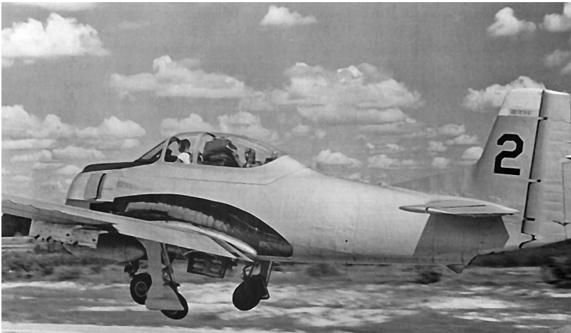
Above: A Water Pump AT-28 takes off from Udorn with a Detachment 6 Instructor Pilot seated to the rear of a student. The inboard pod with .50 caliber machine guns and the outboard rail for rocket pods can be clearly seen. (Photo courtesy of the Air Commando Association.)
