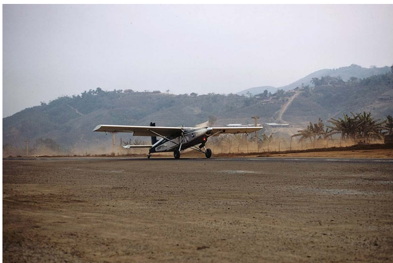
Above: The most preferred aircraft by the Butterfly FAC was the Air America Porter Pilatus, with its ability to operate over north Laos and get into short airfields. (From the collection of William E. Platt, Raven 43.)
