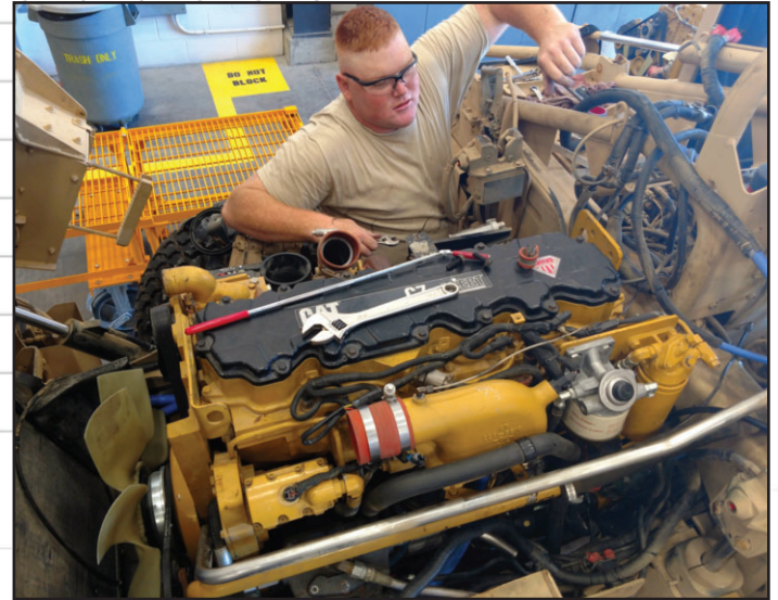
Spc. Taylor Rahe, 995th Surface Maintenance Company, prepares to replace an engine on a Medium Tactical Vehicle during annual training at Camp Dodge, Iowa July 21.
