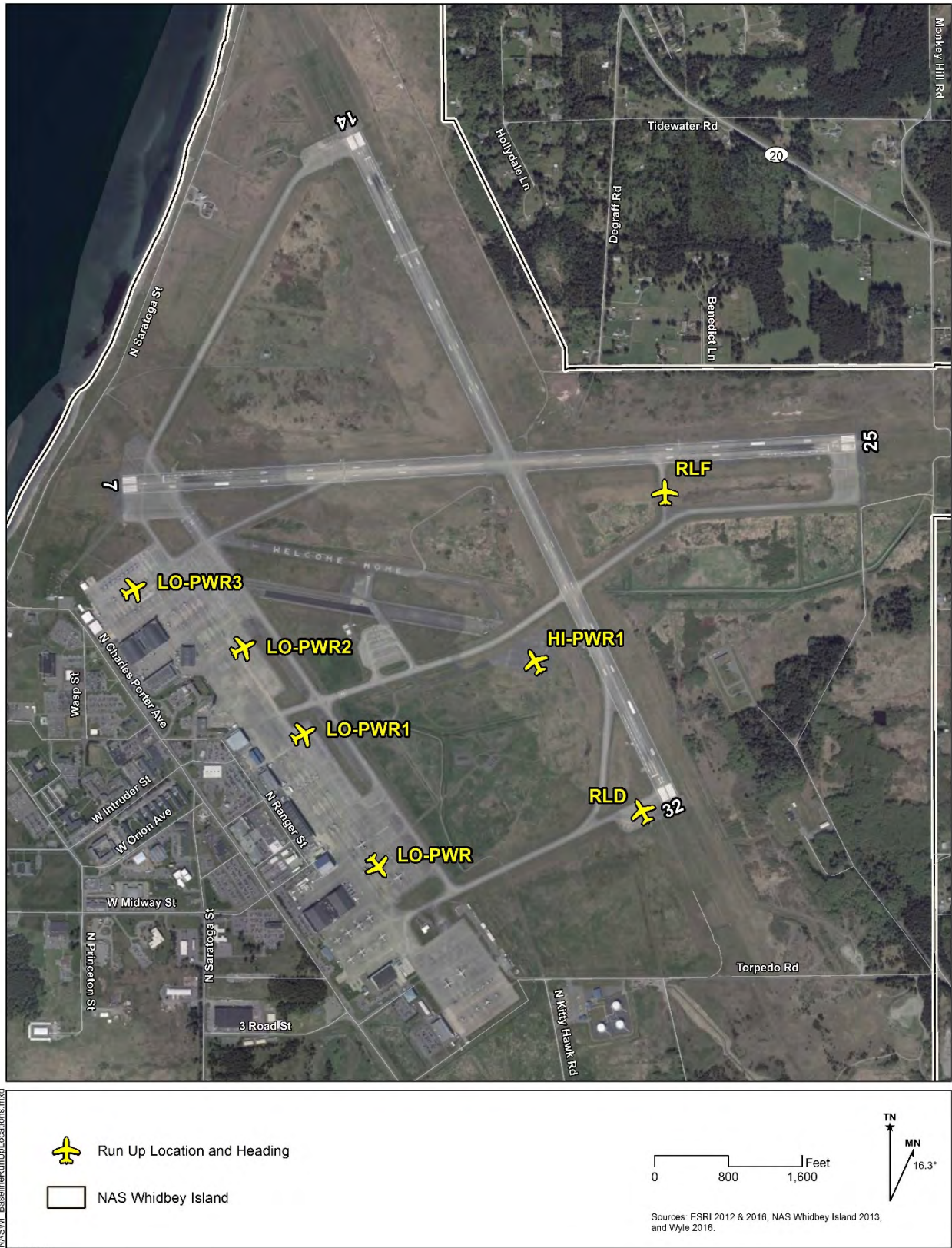
Figure 4-1 Modeled Run-Up Pads For Baseline Scenario
