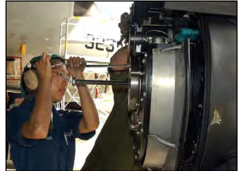
An Aviation Machinist's Mate removes the propeller control of a P-3C Orion for routine maintenance. NAS Whidbey Island's Ault Field has an Aircraft Intermediate Maintenance Detachment (AIMD) and several maintenance and hangar facilities.
