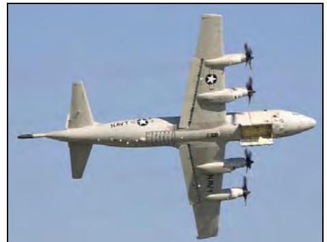
A P-3C Orion flies with bomb-bay doors open. The EP-3E ARIES uses the same P-3 platform, but is easily distinguishable from the P-3C Orion by features such as a dome under the front fuselage and additional "canoe" fairings that cover antennas.
