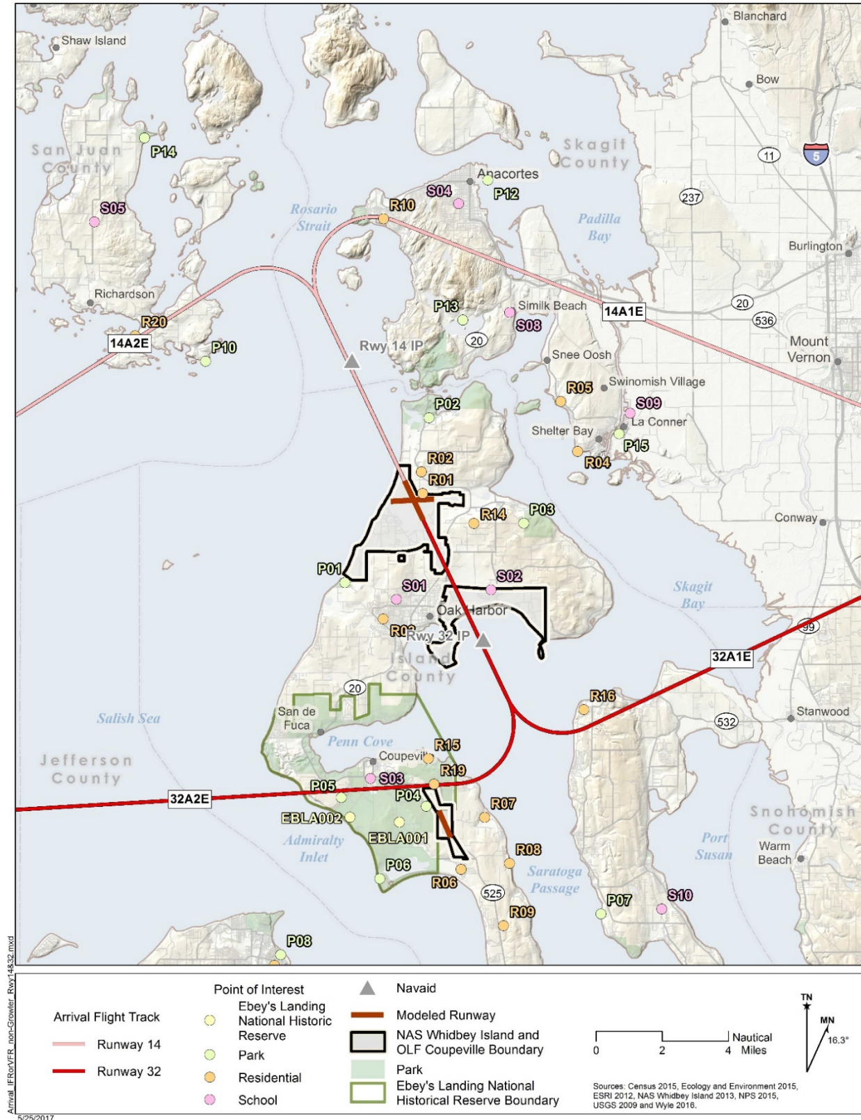
Figure A4-6 Modeled Average Daily Other Arrival Flight Tracks to Runway 14/32 at Ault Field (non-Growler)
