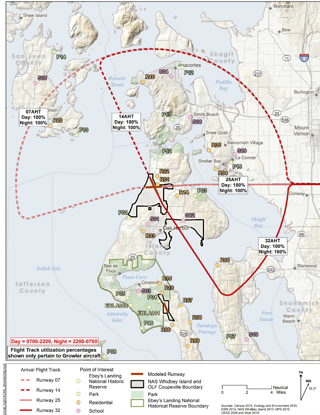
Figure A4-9 Modeled Average Daily High TACAN Arrival Flight Tracks at Ault Field
