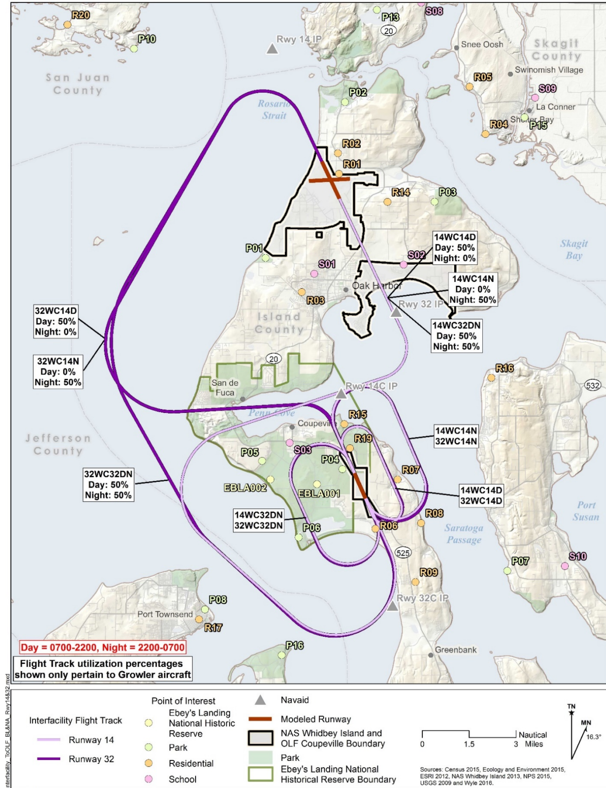
Figure A4-21 Modeled Average Daily Interfacility Flight Tracks from Runway 14/32 at Ault Field to the OLF for Baseline and No Action Alternative
