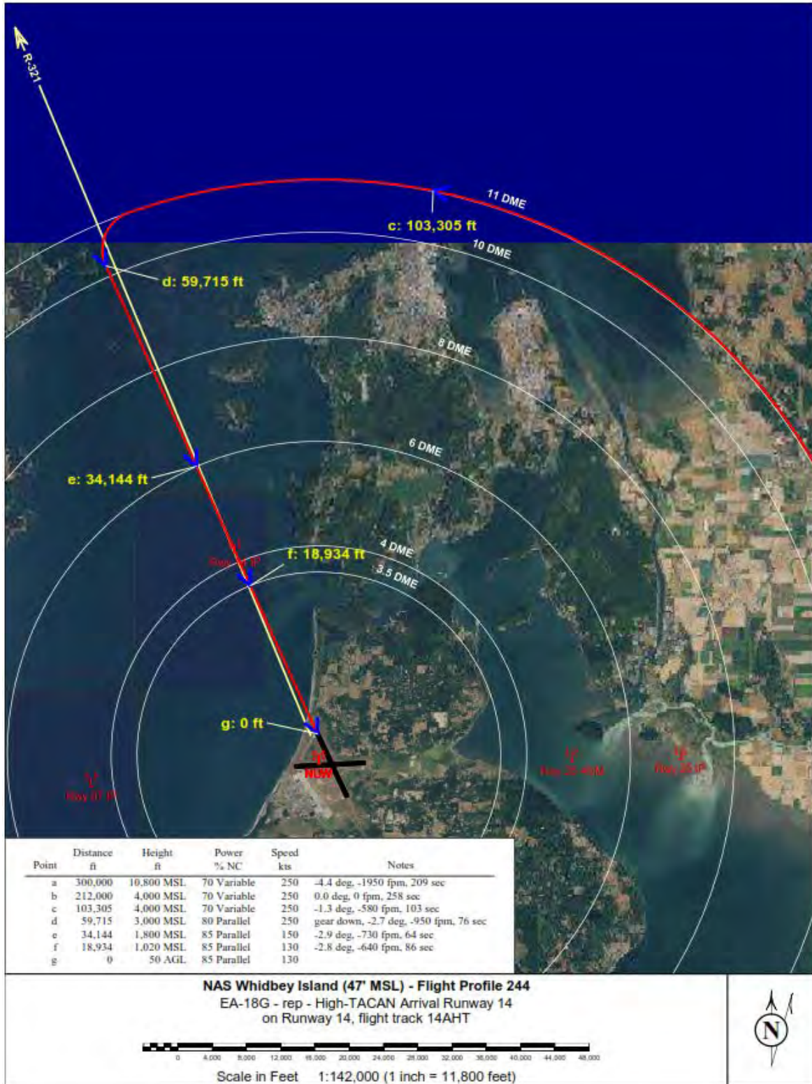
Figure A5-4 EA-18G High TACAN Arrival Flight Profiles at Ault Field Runway 14
