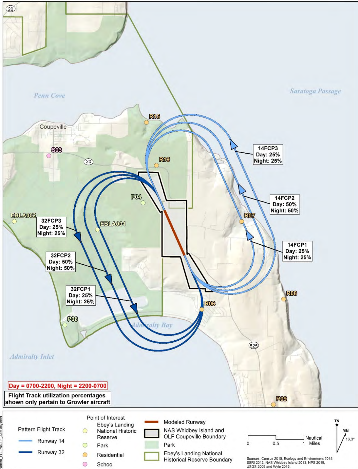
Figure A4-26 Modeled Average Daily FCLP Flight Tracks at the OLF for Numbered Alternatives
