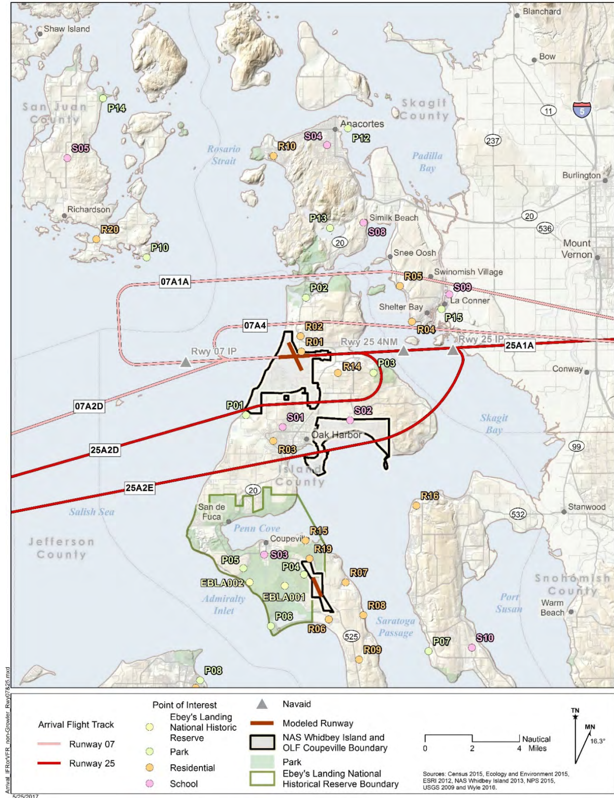
Figure A4-5 Modeled Average Daily Other Arrival Flight Tracks to Runway 07/25 at Ault Field (non-Growler)
