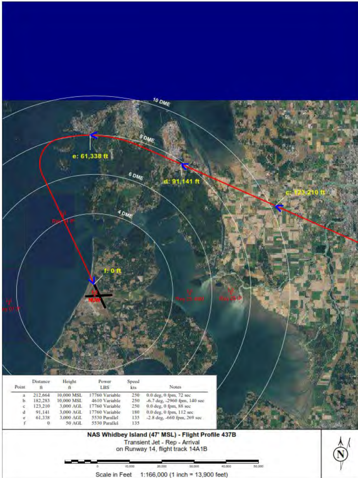
Figure A5-32 Transient Large Jet Straight-in Arrival Flight Profile at Ault Field Runway 14
