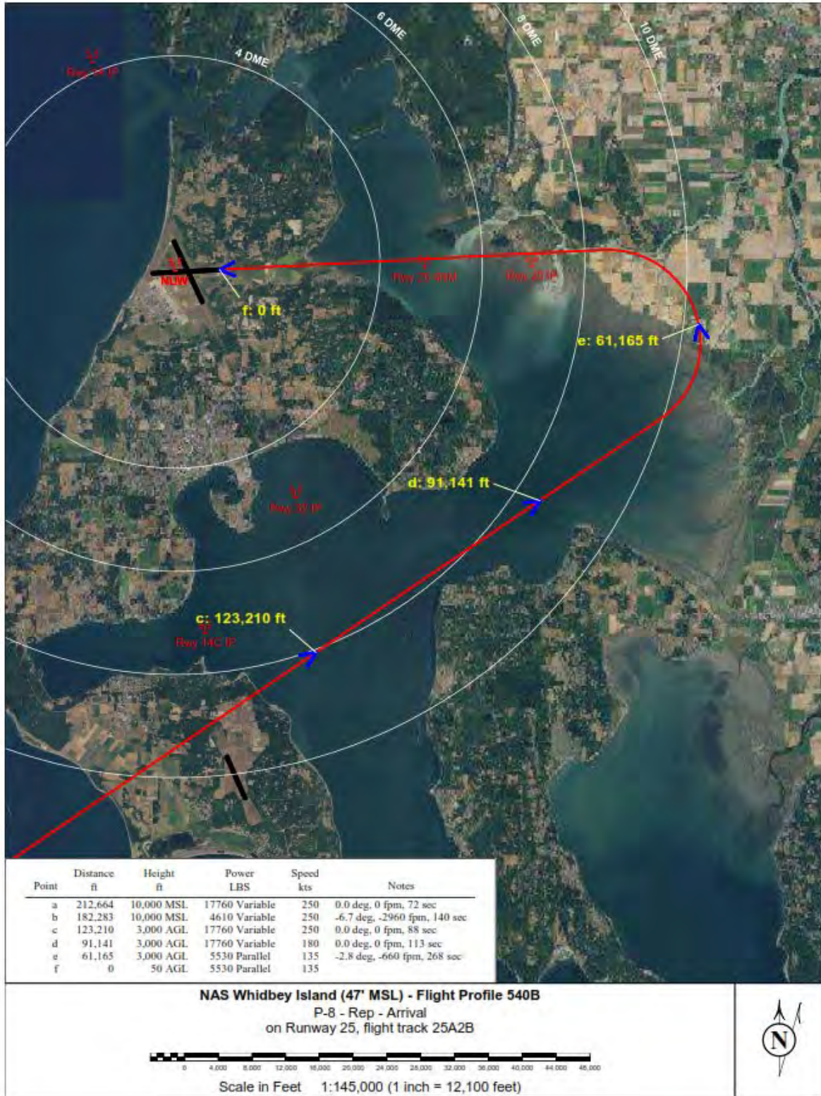
Figure A5-27 P-8A Straight-in Arrival Flight Profile at Ault Field Runway 25 (Longer Final)
