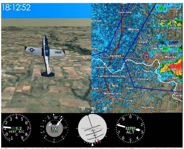
Figure 1: On the left, the MA maneuvering before loss of control effectiveness. On the right, the red circle represents the approximate aircraft location. Time is represented as Greenwich Mean Time (Tab NN-2).
