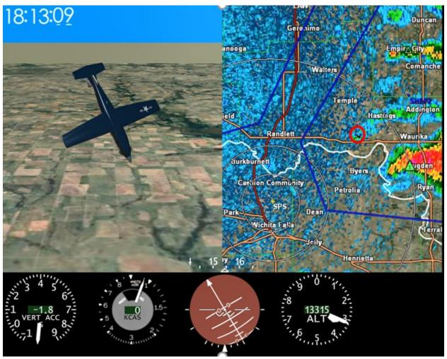
Figure 3: The left depicts the MA established in spin. The red circle on the right represents the approximate aircraft location. (Tab NN-2)
