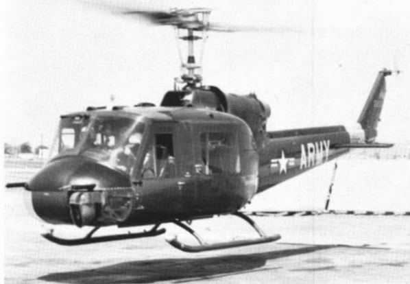
TOW SIGHT —Army UH-1B helicopter takes off on accuracy test of experimental sight for launching TOW missile.
