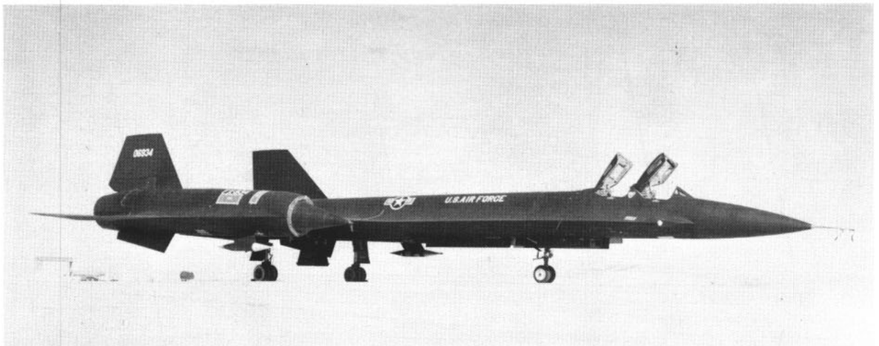
EXPERIMENTAL JET—YF-12A, capable of sustained 2000-mph flights, is being tested as a long-range interceptor.
