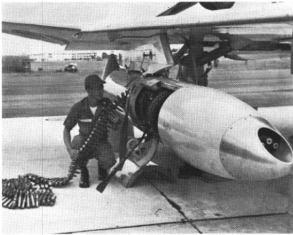
AMMUNITION is loaded into test gun pod on AF F4C Phantom. Pod's 20-mm gun fires 6000 rounds a minute.
