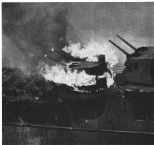
JETS OF FIRE envelop five-inch gun mount. Men in Santa Fe fought blaze by aiming hoses through hatch at rear.
