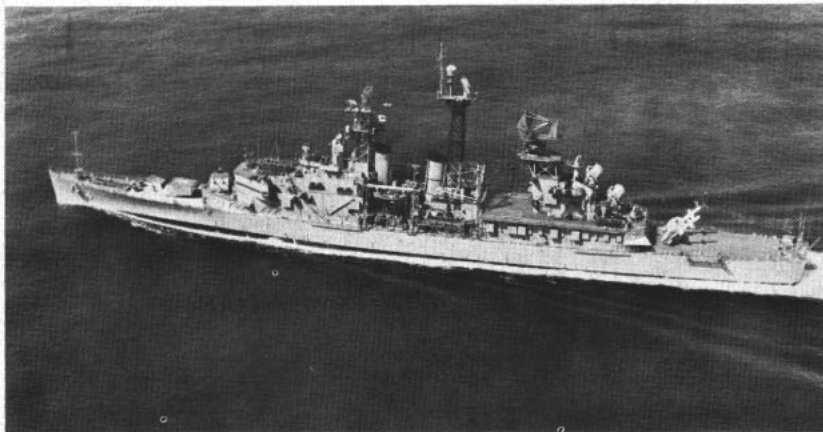
NO LIGHTWEIGHT — The 10,670-ton guided missile light cruiser uss Little Rock (CLG 4), formerly (CL 92), is equipped to fire Talos guided missiles.
