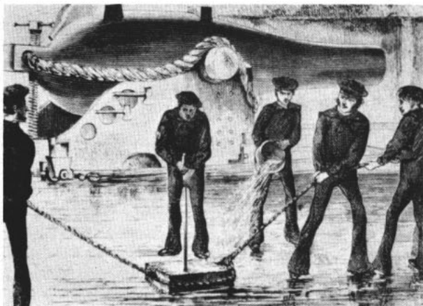
STONING — Even old-timers probably won't recognize this type holystone used to clean the wooden decks.
