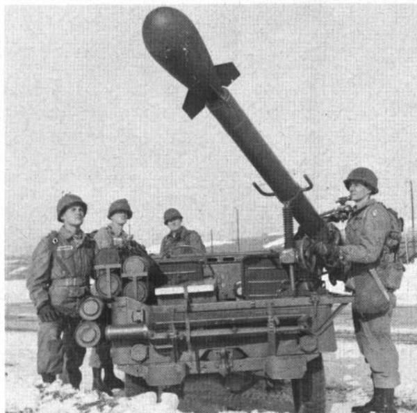
NO BEAR GUN—Army's Davy Crockett, a hand- or jeep-portable weapon, fires conventional or atomic warhead.
