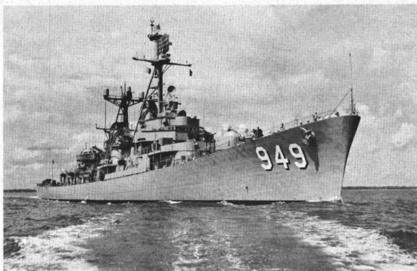
BACKFIRING — The destroyer USS Parsons (DD 949) is one of the first U.S. warships with guns arranged to provide more firepower aft than forward.
