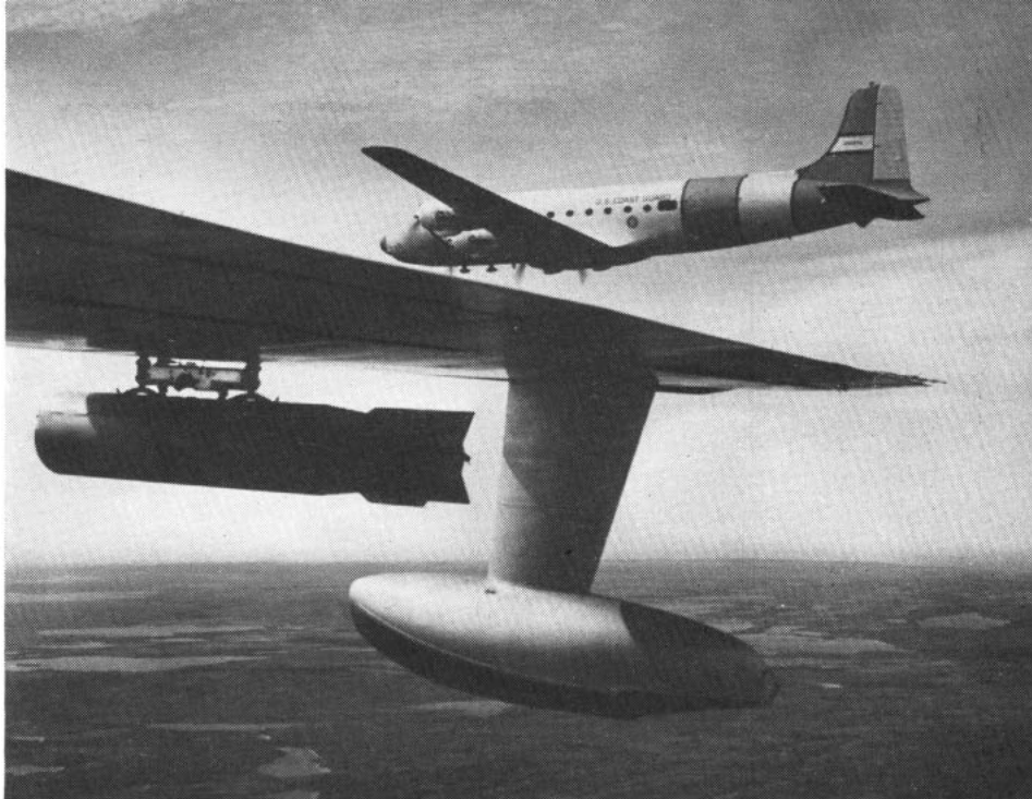
HOT SHOT —Coast Guard plane carries thermite bomb for test on heat destruction of bergs. Below: Radar on patrol plane helps spot dangerous ice.
