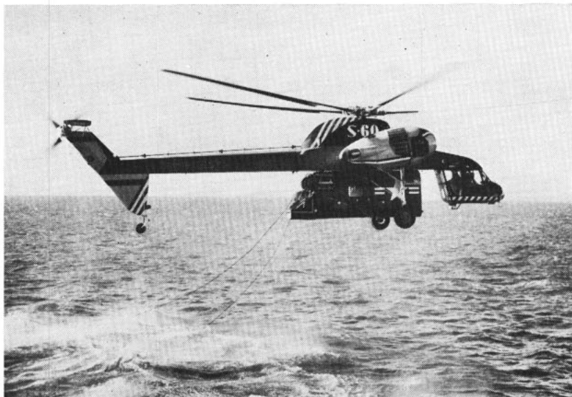
WHAT IN THE WORLD —Weird looking copter is a skycrane with new light-weight minesweeping gear. Here it demonstrates its sweeping techniques.
