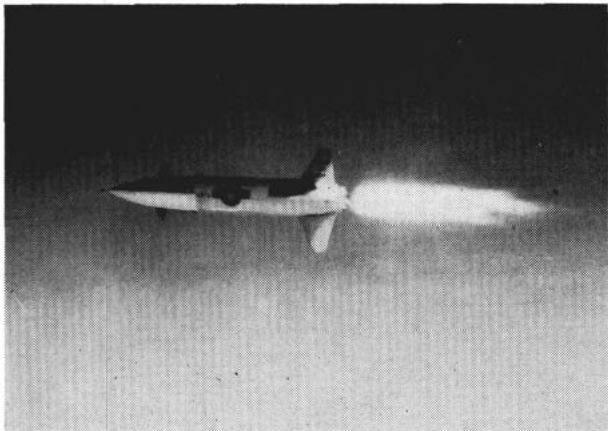
RASCAL, long-range rocket-powered missile, is built to be released in flight, proceed at high speed to target.
