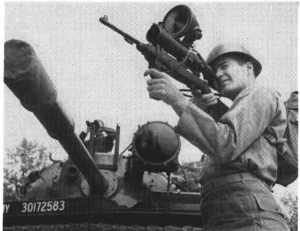
IN THE RED—Army men and tanks gain night mobility through infrared sniperscopes and tank searchlights.
