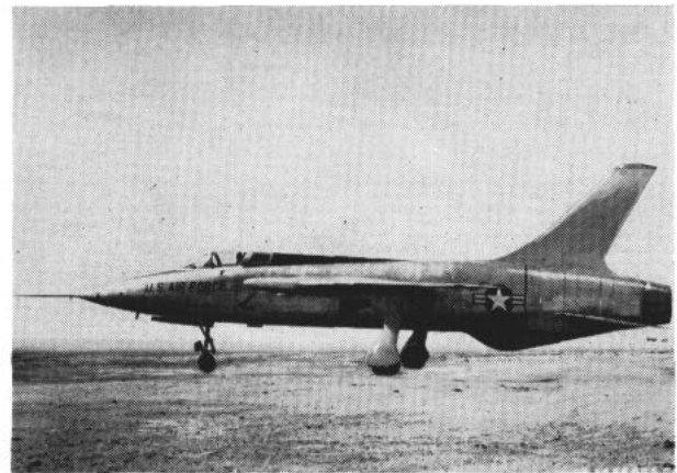
AIR FORCE'S new Thunderchief F-105 with needle-nose radar unit is latest thing in supersonic fighter-bombers.
