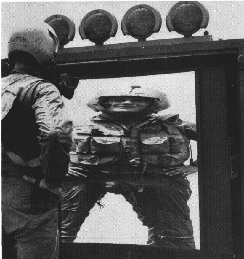
MIRROR TRICK —The optically ground concave surface may reflect some wierd sights, but it is also credited with reducing landing accidents by one third.
