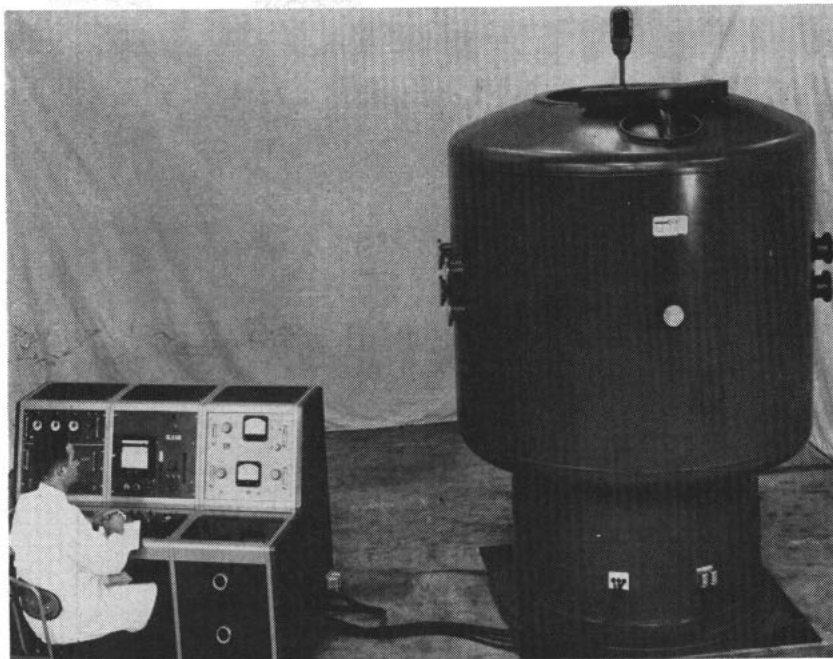
NUCLEAR REACTOR —Super safe atomic reactor, designed to produce just enough power for flashlight bulb, will be used at Naval Post Grad School.
