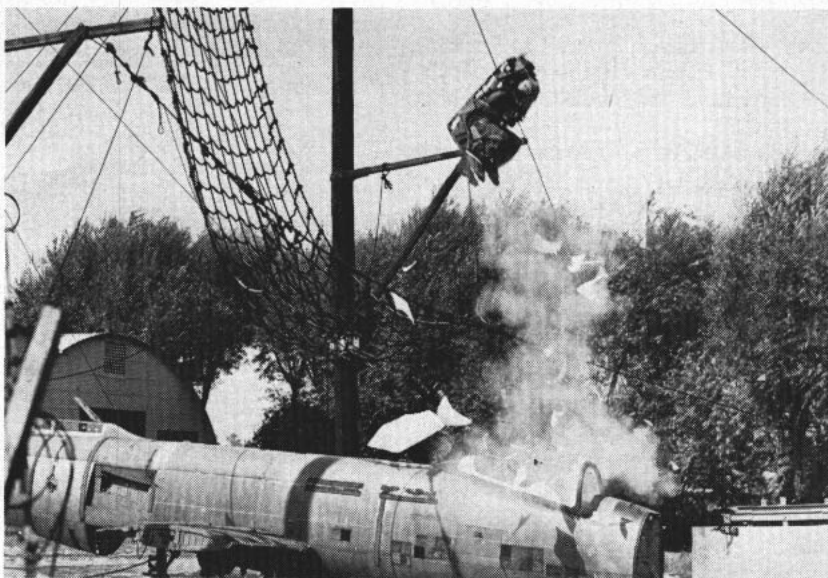
PILOT HURTLES skyward in test of canopy ejection seat. In emergencies, fliers can be ejected quickly and safely from jet planes by means of new system.
