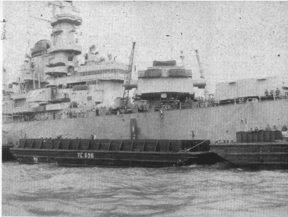
OPEN LIGHTER (YC) takes ammunition from USS Missouri (BB 63). Navy has 16 kinds of lighters, ranging from cargo and garbage to 'special purpose.'
