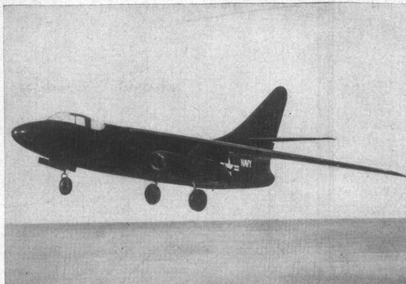
ATTACK BOMBER built for carrier operations, the X-3D will fly between 600 and 700 mph. Model shows under-wing position of the jet's powerful engines.
