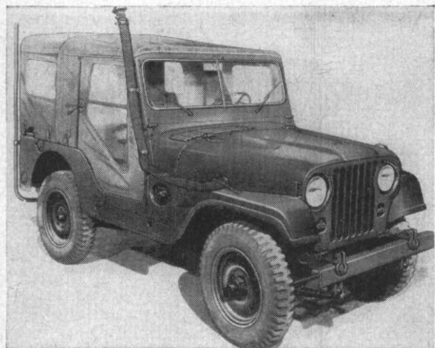
DEEP BREATHING JEEP that can travel underwater has been perfected and ordered into production by the Army.
