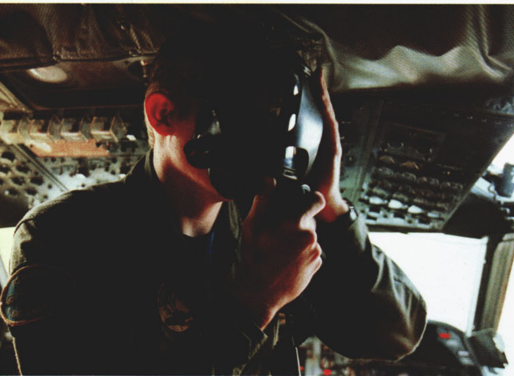
AE2 Dale Dennison checks the airways for all of the masks before flight. In the unlikely event the aircraft should lose cabin pressure, the masks are close by and ready to use.
