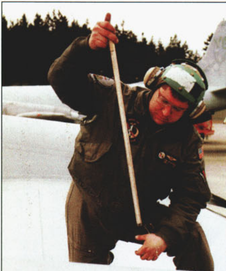
AME2(NAC) Bob Renfrew, with Wing 10, checks the fuel quantity on each side of the aircraft's wings. "I love my job," said Renfrew. "A lot of people count on me to do my job right the first time, every time."
