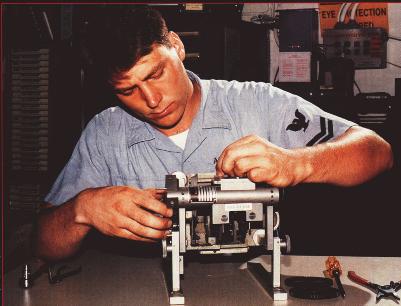
On board USS George Washington (CVN 73), AO2 Brian Ashworth, a member of Reserve Unit 291, sets the timing of an ejector assembly of an M-61A1 20mm Gatling gun. The Gatling gun fires 600 to 800 rounds per minute, has a capacity of 1,800 rounds and adds about 900 lbs. to the F/A- 18 Hornet .
