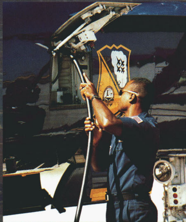
AD1(AW) Foster Stringer, of Birmingham, Ala., services a Blue Angel F/A-18 with smoke oil before a demonstration.
