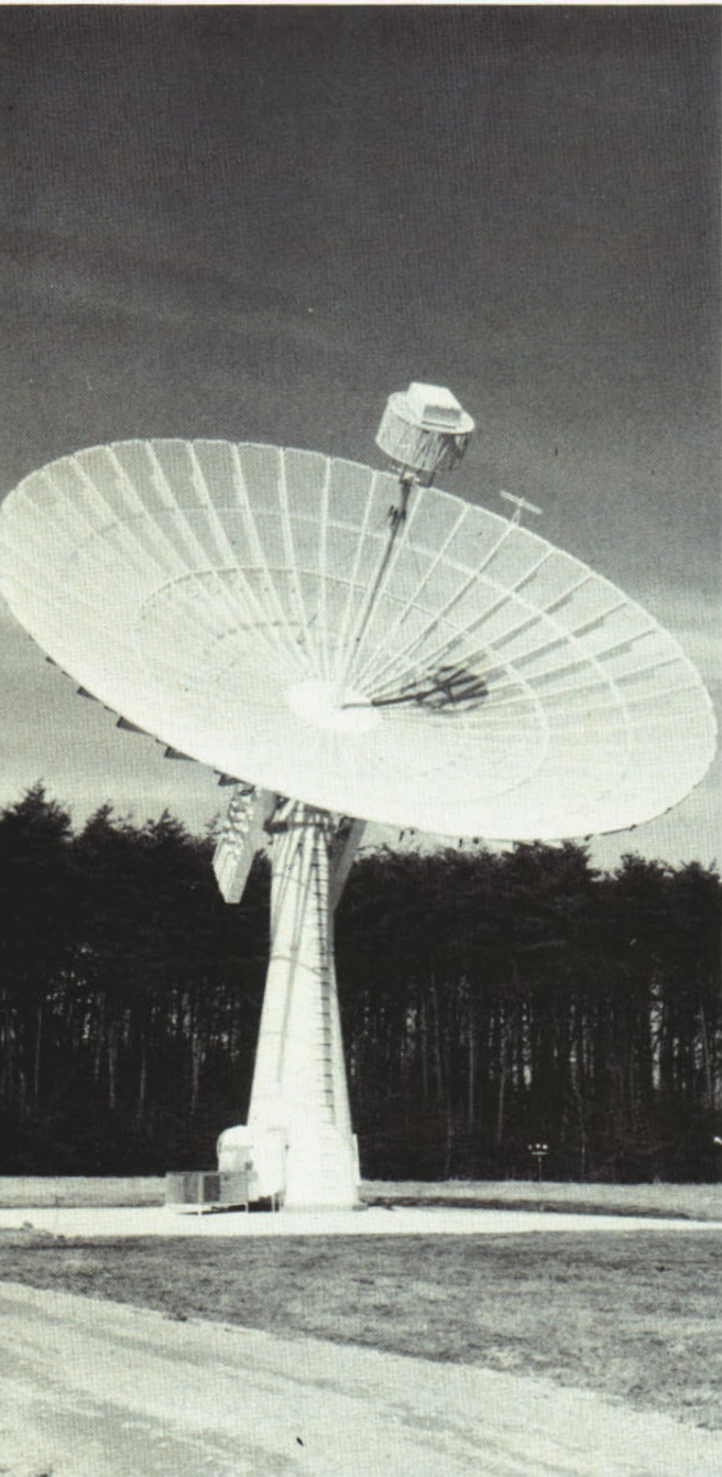
A 48-foot telemetry antenna to be used for tracking the SOLRAD spacecraft.
