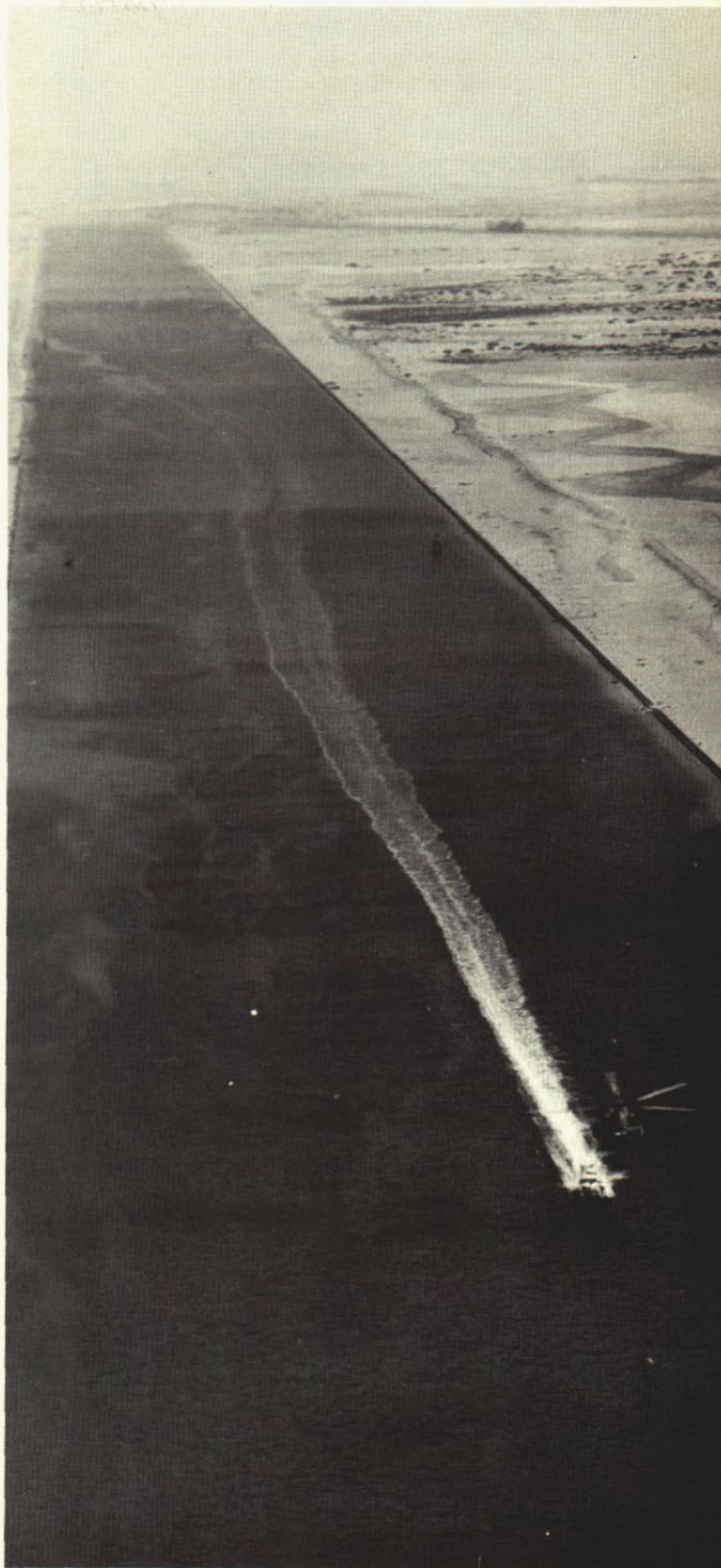
Left: Helicopter Combat Support Squadron Six helicopters practiced their normal role by flying supplies from Ismailia to the LST flagships on Lake Timsah. Right: An RH-53D Sea Stallion helicopter tows a magnetic minesweeping sled on the Suez Canal.
