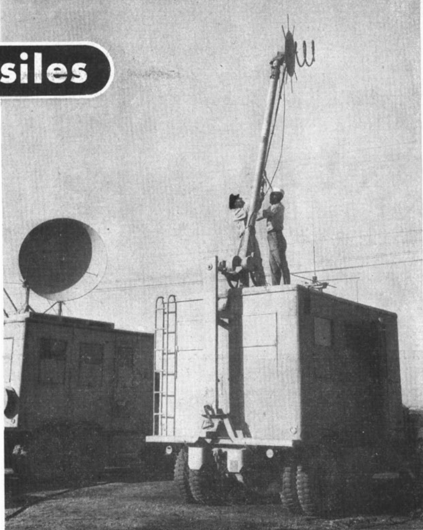
ANTENNA on telemetering van is hoisted into position by students. Telemetering is used to obtain data transmitted from the missiles in flight.
