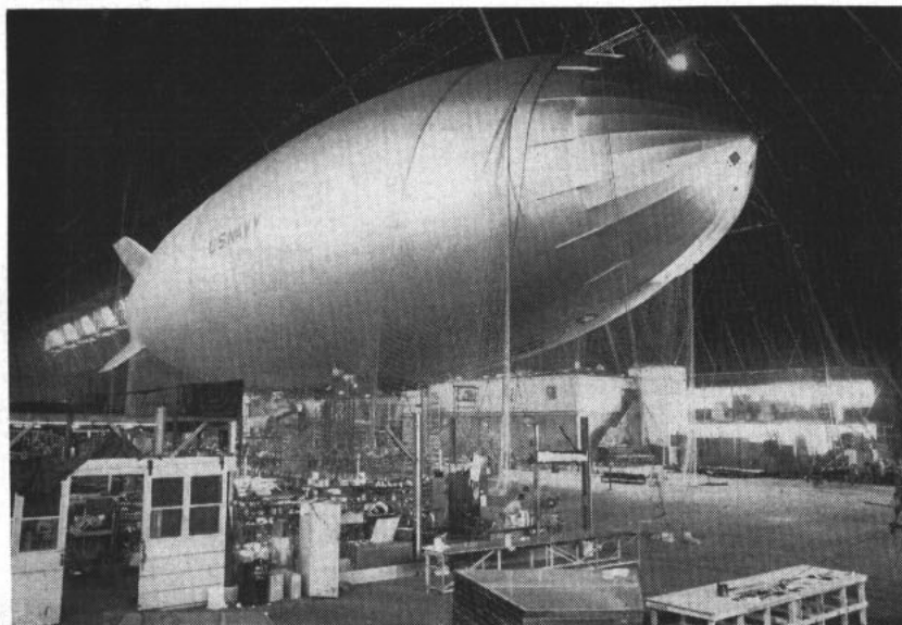
LARGEST non-rigid airship ever built, the Navy's new N-type antisubmarine blimp is held secure by huge net while its gondola is attached at Akron, Ohio.
