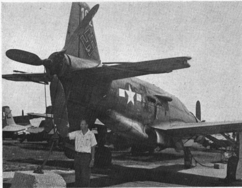
FANTASTIC Nazi bomber, the Dornier 335, has power coming and going—she has engines in nose and tail. It too is being fitted for a plastic overcoat.
