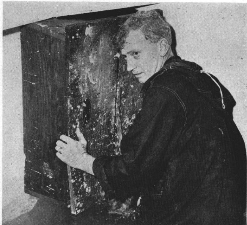
SHELL HOLE in Buttercup's battered bulkhead is plugged temporarily by a mattress stuffed in a box and held by an anxious trainee until shores are cut.
