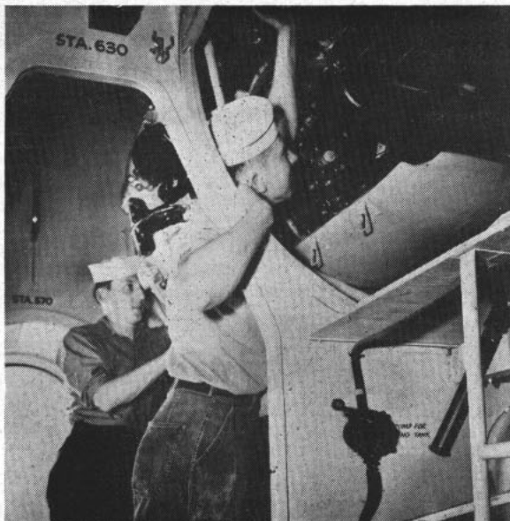
ENCLOSED engines make possible repairs while in flight (left). Right: 'Joe' is served in upper deck galley of mock-up.
