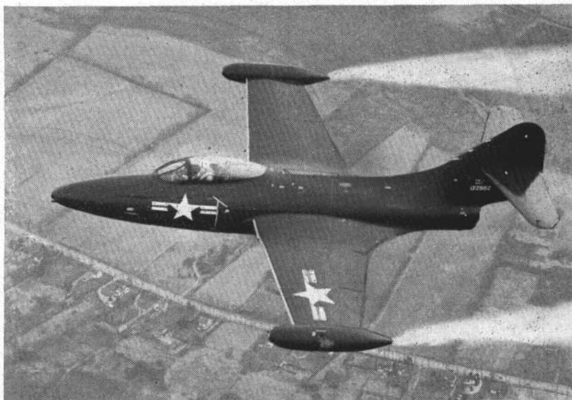
NON-DROPPABLE wing tanks on Navy's F9F-3 Panther have provision for jettisoning fuel in less than 40 seconds. Plane's speed eliminates fire hazard.
