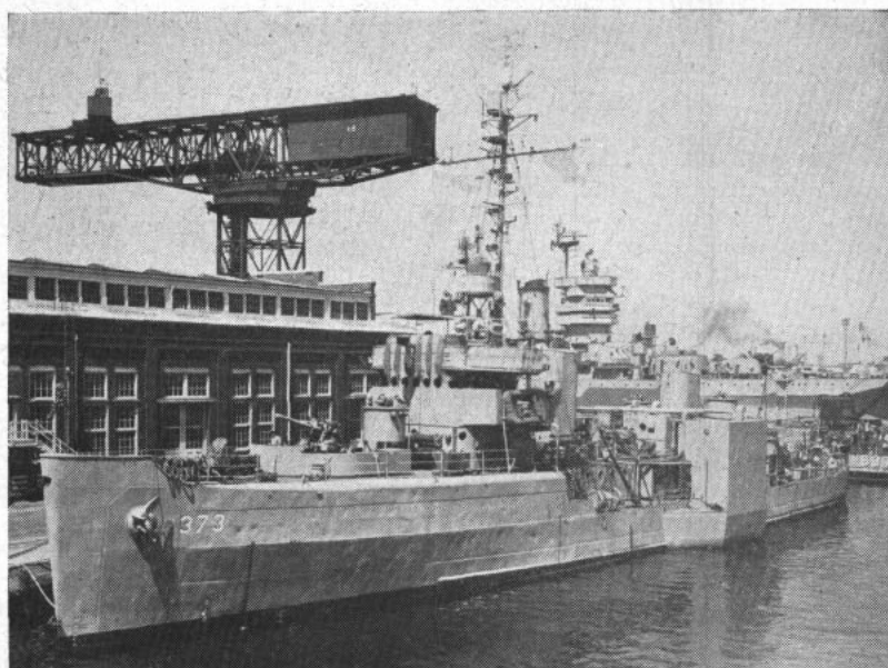
BOX-LIKE stabilization system, attached outside the hull of Peregrine to minimize structural changes, is designed to reduce her roll by 80 per cent.
