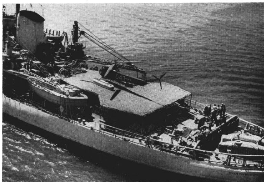
ICE BREAKERS use helicopters for rescue work and general reconnaissance. The restricted flight deck is ample even when the ship is under way.
