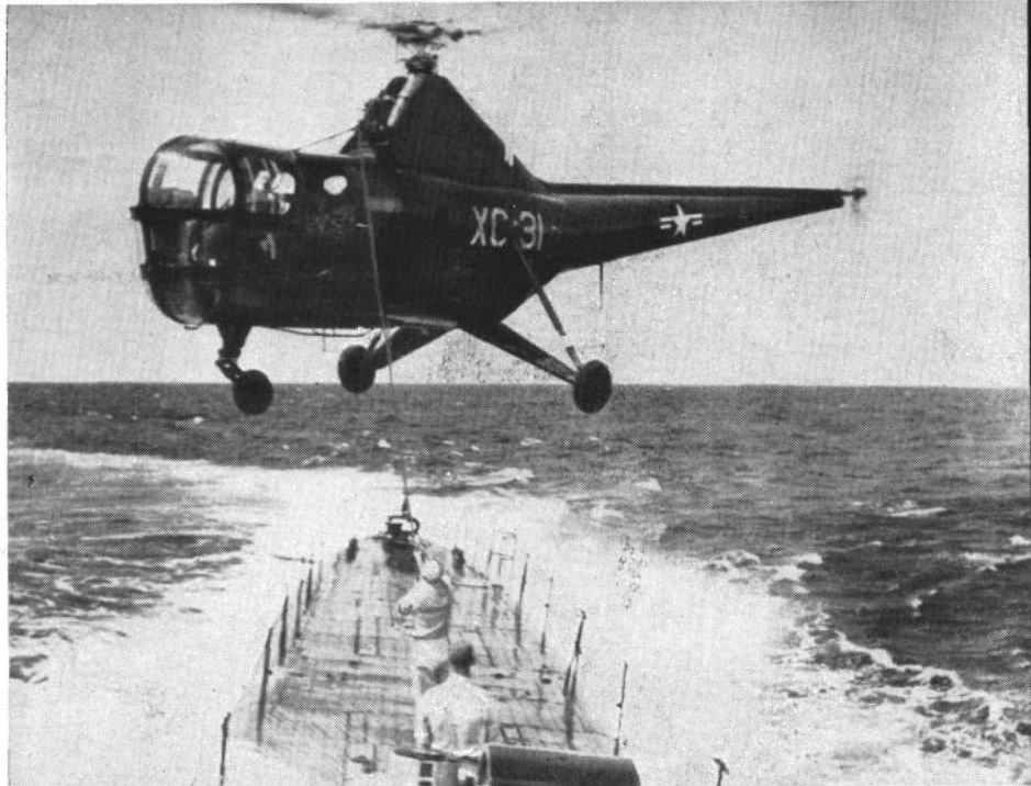
TAXI SERVICE technique is demonstrated by the current fleet wheel horse, the HO3S-1. Hovering, it raises and lowers personnel by means of hoist and sling.
