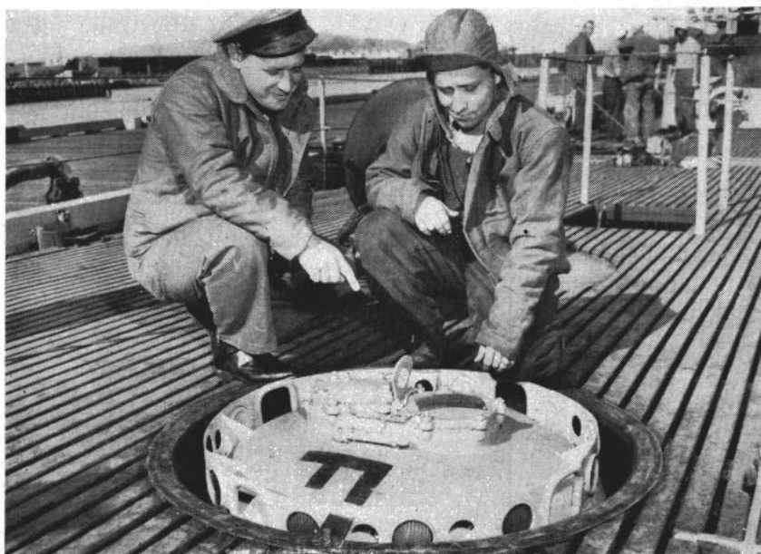
OLD TYPE buoy contains no mechanism for hauling down the rescue chamber.
