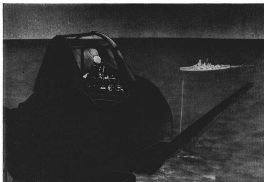
TORPEDO ATTACK trainer developed by the Navy uses actual combat films to train student pilots under realistically simulated battle conditions.
