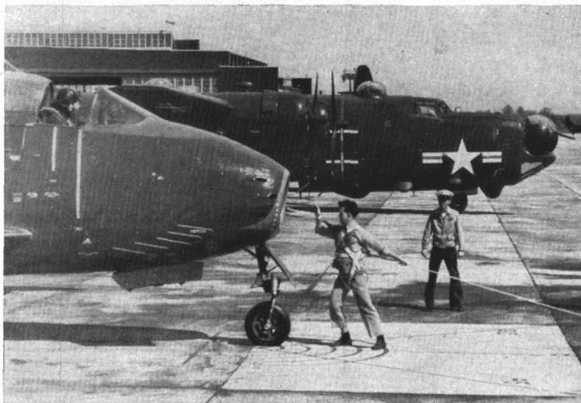
SUCTION of an FJ-1 jet turning-up at full power is being tested by a volunteer at NATC Patuxent River to determine the forward danger area.
