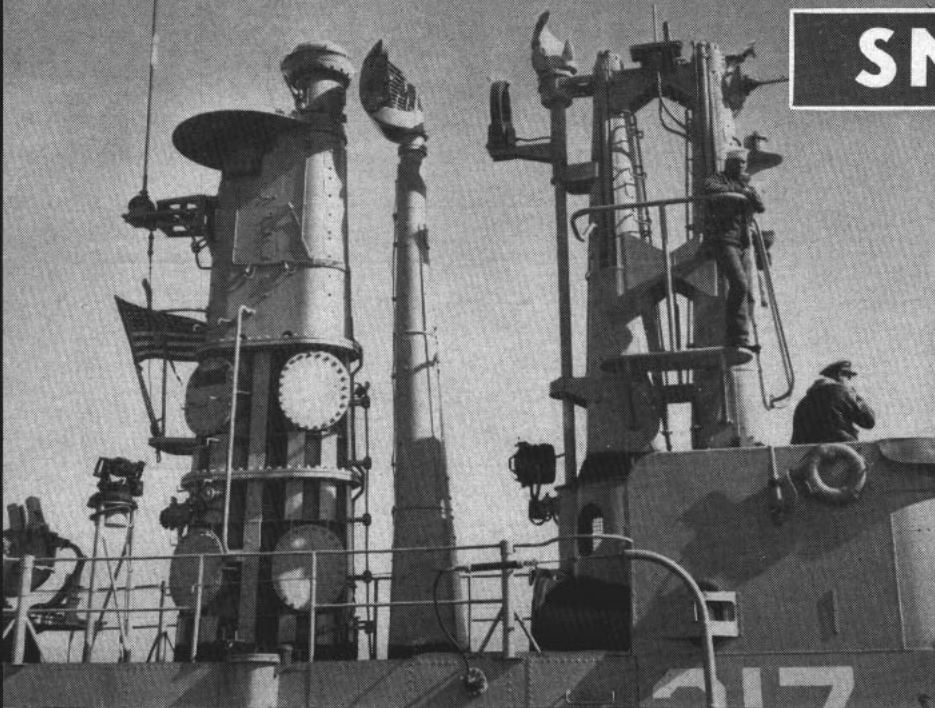
SNORKEL shears of USS Barbero are visible at left. Device enables 'submarines to cruise at nearly full periscope depth for extended periods of time.
