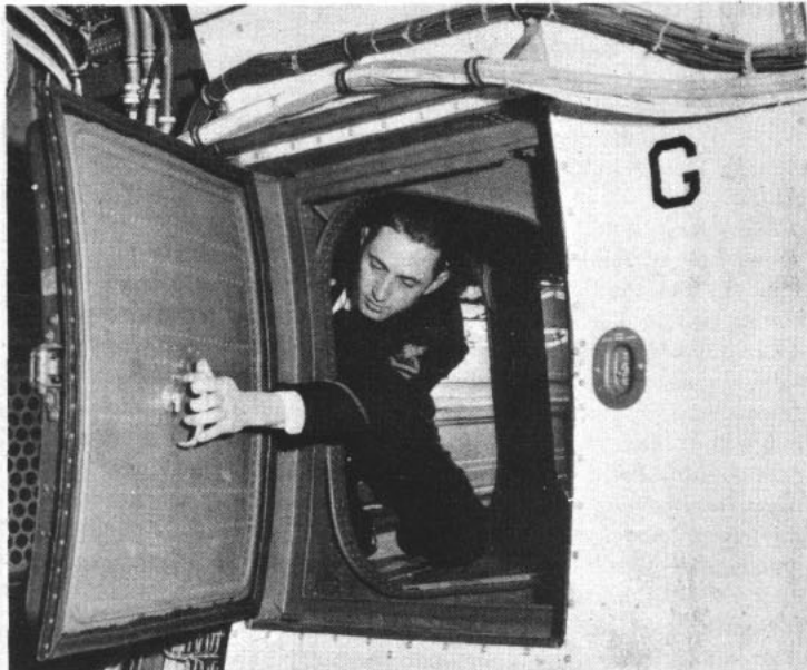
LARGEST Navy transport plane Constitution seats 92 passengers in upper deck (left). Wing tunnel leads to engines.
